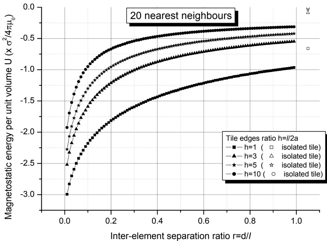
**Fig.2:** Magnetostatic energy per unit volume vs. inter-element separation ratio for different tile edges ratio considering inter-tile interactions up to 20 nearest neighbours. In Co, for example,  $\sigma^2/4\pi\mu_0 \approx 2 \cdot 10^5$  J/m. For comparison purposes, the magnetostatic energy of an array of isolated elements, i.e., infinite separations, is also displayed.
