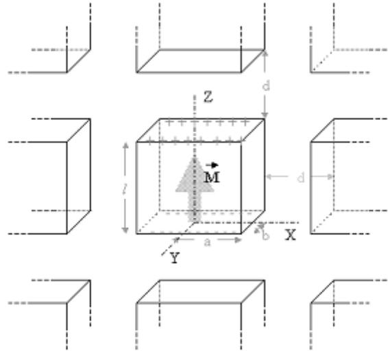
**Fig.1:** Problem conditions: The magnetization lays parallel to the tile edge, creating two magnetic poles surfaces of area  $2a \times 2b$ . Tiles are separated a distance  $d$  both in the  $X$  and  $Z$  directions.
