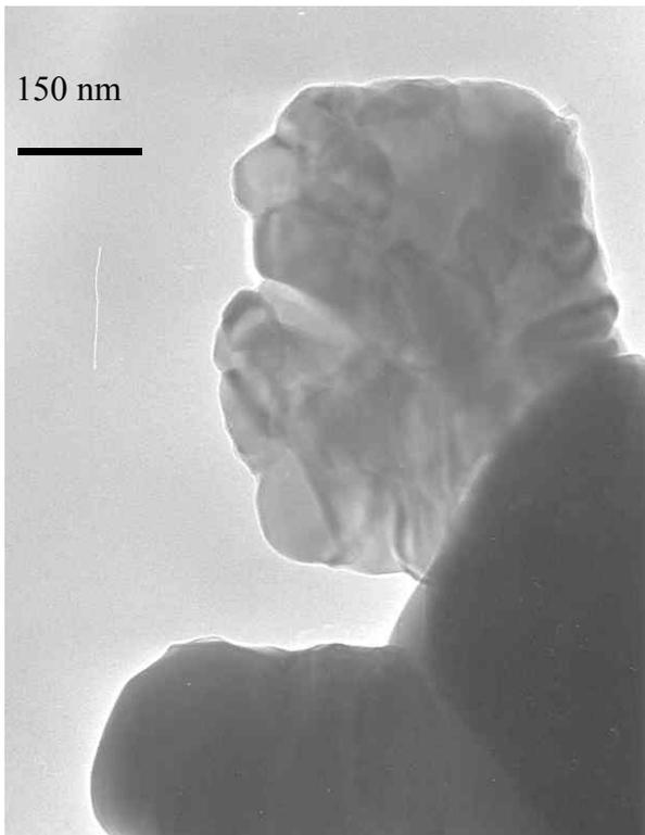
Fig.1 New phase observed after annealing ZnO and MnO<sub>2</sub> powders at 500°C
