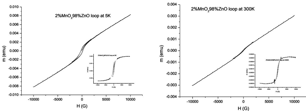
Fig.2 Hysteresis loop at 5 and 300K of 2%MnO<sub>2</sub> 98%ZnO ceramics powders heat treated at 500°C. The insets show the result of subtracting the paramagnetic component from the loops
