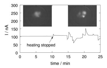
Figure 1. Trace of the emitted current of N-doped nanotube as function of time. The recording started with a stable emission obtained at a temperature of 800 K and an extraction voltage of 359.6 V. Current fluctuations occurred after the heating was stopped as shown at the right side of the plot. The corresponding emission patterns during and after heating recorded with a micro-channel plate and a phosphor screen positioned 1.5 cm in front of the emitter are also shown as insets.
