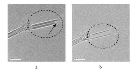
Figure 2. *In-situ* transmission electron microscopy of a degradation reaction of a multi-walled carbon nanotube under the influence of a strong electric field. (a) The open end of a multi-walled nanotube (see arrow), that had been broken-off before, imaged while emitting 8 µA of current at 350 V extraction voltage. (b) The inner walls of the nanotube were removed/destroyed (encircled) and the nanotube continued emitting current of 3 µA at 360 V.
