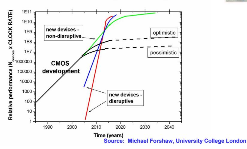
CMOS: Limits of scaling & limits of benefits of scaling: frequency increase, power scaling, delays, etc.
