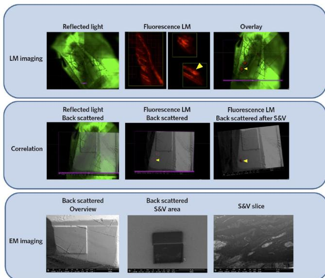
**Fig. 1** > Images taken throughout the experiment. The top row shows images from the light microscope, and the bottom row shows images taken from the DualBeam. The middle row shows the overlays between the LM and EM images used to correlate. The yellow arrowhead indicates the cell followed throughout the workflow./
