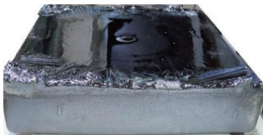
Fig. 1 > Photograph of the silicon ingot grown with the optimum conditions observed in the current study./
