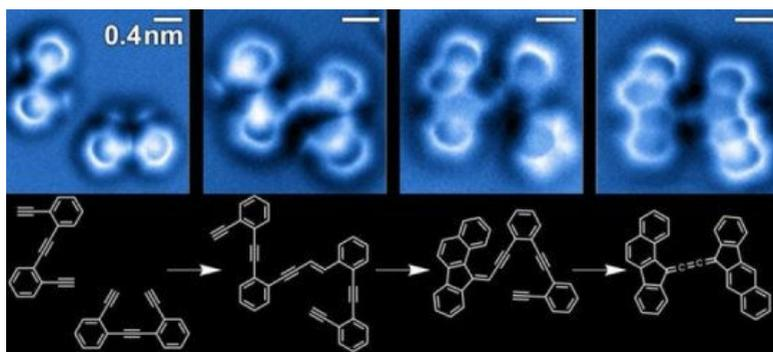
**Fig. 1** > Sequence of images of the steps in the reaction of enediyne molecules on a silver surface. (A. Riss / Technische Universität München.)
