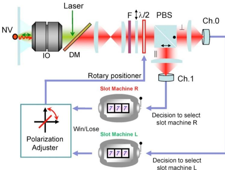
**Fig. 1** > System architecture for single-photon decision maker and schematic diagram of experimental setup./
