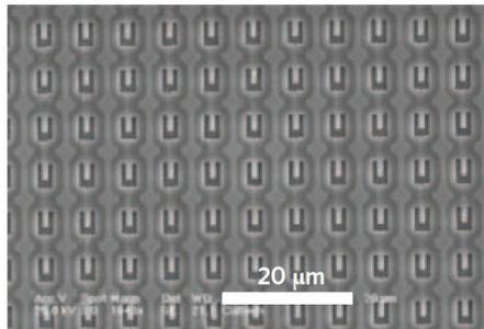
**Fig. 10** > (Left) Resonance spectrum of a single mechanical resonator. The quality factor of the device is unaffected when the channel is filled with water (red line). (Right) Array of silicon cantilevers [5]./
