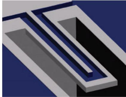
**Fig. 9** > [5] (Left) Schematic of static-mode surface-stress sensing MEMS device. (Right) Suspended microchannel resonator (SMR). The fluid containing the target molecules flows through a channel inside the device and binds to the inner flow-channel walls, while the resonator oscillates in air or vacuum./
