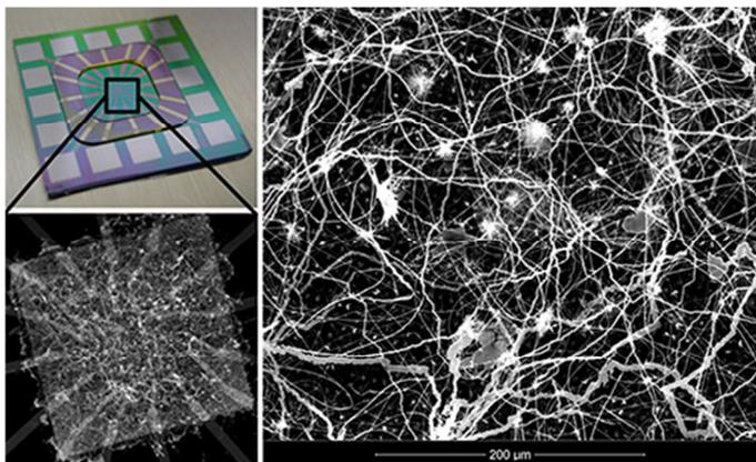
**Fig. 1** > A look inside the ASN device reveals its highly interconnected architecture which comprises synaptic circuit elements at each point of contact between nanowires. The collective interactions between these atomic switches result in unique, emergent properties which have shown significant potential for neuromorphic computing./
