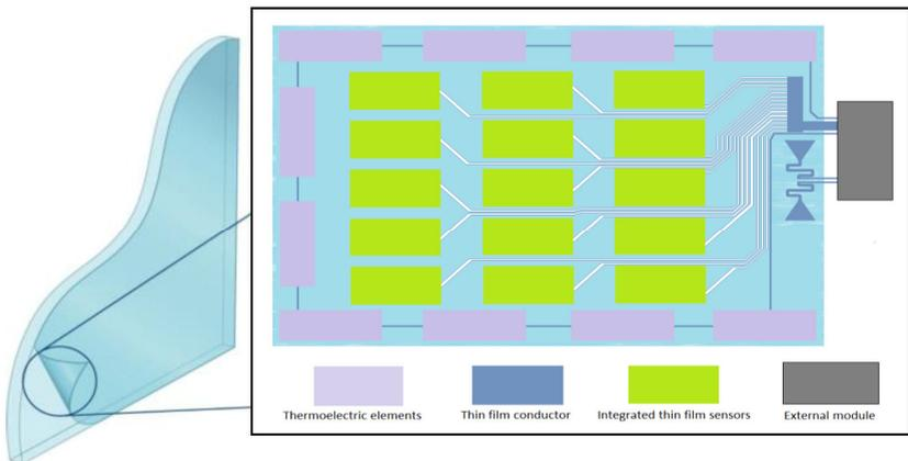
Fig. 3 > Integration of thermoelectric modules, thin film sensors and external control module in a smart window application./
