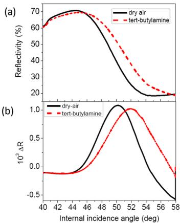
**Fig. 2 >** Angular measurements of the Reflectivity (a) and TMOKE signal (b) under Kretschmann configuration which allows SPP excitation for the ZPD functionalized MO-SPR sensor with dry-air (black continuous lines) and tert-butylamine vapours (red dashed lines) inside the gas chamber./
