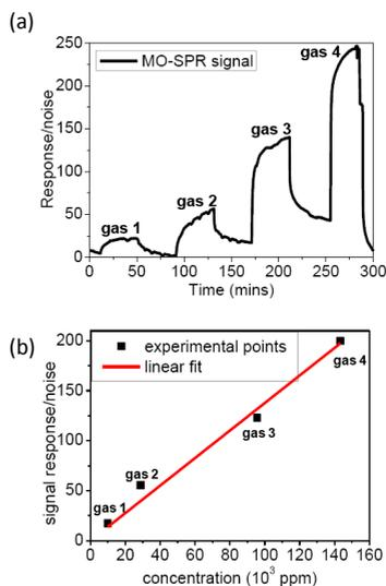
**Fig. 3** > Sensorgram (a) and calibration curve (b) of the ZPD functionalized MO-SPR sensor for four different concentrations of VOC vapours. A linear fit is also presented for the tert-butylamine detection./
