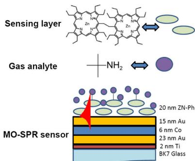
**Fig. 1** > Sketches of the molecular structure for both the ethane-bridged Zn-porphyrin dimer (ZPD) as sensing layer and the tert-butylamine as gas analyte. Besides, a scheme of the ZPD functionalized MO-SPR sensor detecting the organic vapours is shown at the bottom of the figure./
