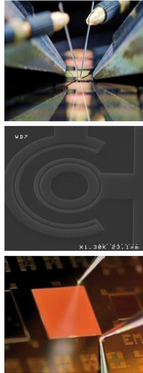
**Fig. 15 >** Top: a silicon photonic integrated circuits with active emitters for electrical driven Er coupled to Si-nc optical amplifiers. Centre: an electrical driven active optical resonators. Bottom: a CMOS LED with emitting silicon nanocrystals. (Courtesy of Pavesi et al, UNITN and LETI unpublished data)./
