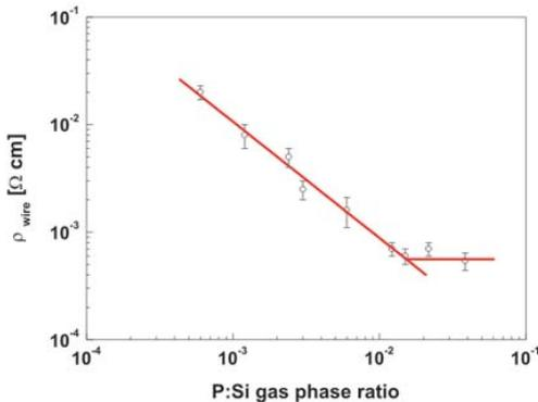
Fig 34. Experimental data of nanowire resistivity vs phosphine concentration. Donor densities up to the solid solubility limit of phosphorous in silicon was achieved.
