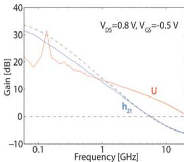
Fig 32. Measured and modelled RF gains for a 90 nm gate length InAs MOSFET.
