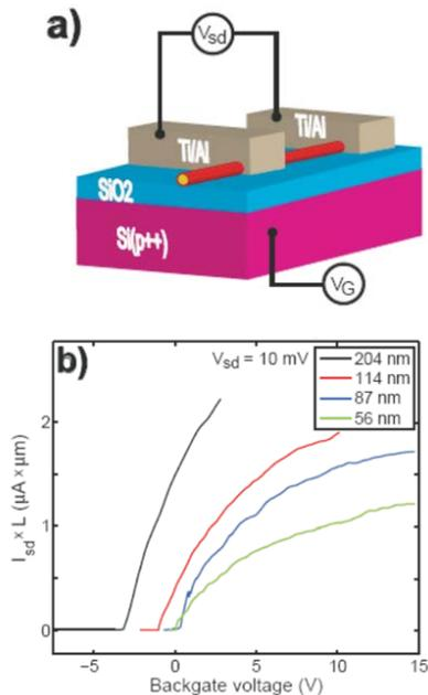
**Fig 2.** (a) Schematic of a Ti/Al contacted nanowire on a heavily doped Si substrate with SiO<sub>2</sub> dielectric. (b) Current through the nanowire as a function of backgate voltage for several NW diameters. Such measurements are used to determine the electron mobility.
