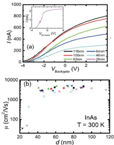
Fig 24. (a) The backgate sweeps for different sections within the same nanowire. The inset shows the data for the section with the smallest diameter. (b) The mobility determined from backgate sweeps. Different symbols correspond to the different devices studied.
