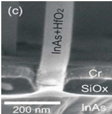
Fig 14. Cross section of the MOSFET, showing the 50 nm Cr gate around the InAs nanowire.
