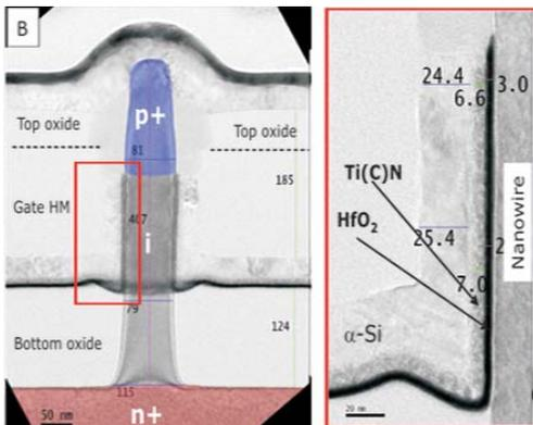
Fig 18. Cross section of the vertical TFET featuring 3nm  $\text{HfO}_2$ , 7nm TiN and 25nm a-Si gate stack around the nanowires.
