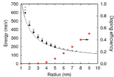
Fig 30. Binding energy of various donors (black symbols, left axis) as a function of the radius R of silicon NWs in vacuum, and room temperature doping efficiency of P donors (red symbols, right axis). The doping efficiency rapidly decreases below R = 10 nm.
