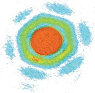
Fig 29. Coherent diffraction of single 95 nm Si nanowire (111) Bragg reflection. The “ab initio” analysis of this pattern allows reconstructing the shape of the NW.
