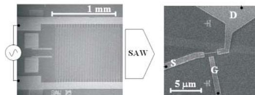
Fig 23. Sketch of the device and set-up for the induction of acoustoelectric current in NW FETs.
