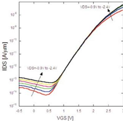
Fig 42. Input  $I_{ds}$ - $V_{gs}$  characteristics of the n-TFET device with an epi grown P<sup>+</sup> source and a nanowire size of 50 nm on design.
