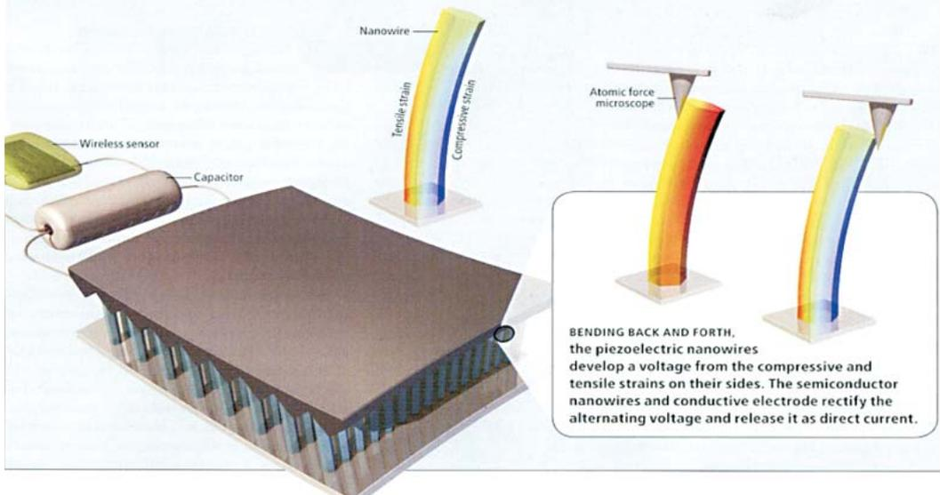
Schematic of piezoelectric energy conversion with nanowires.
