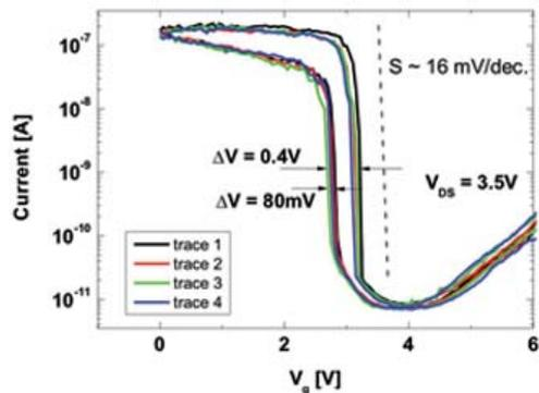
Fig 20. Stability of the transfer characteristics of a vertical IMOS FET.
