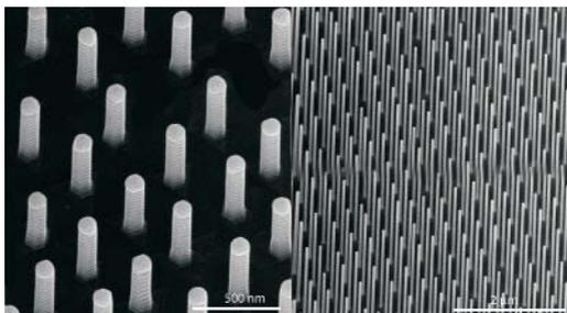
Fig 1. Scanning electron micrographs of gold particle-assisted, MOVPE grown, InAs nanowires in regular arrays, where the positions of the gold particles have been defined by electron beam lithography.
