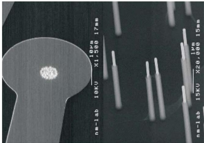
Fig 4. Scanning electron micrograph of nanowire-based electrodes.
