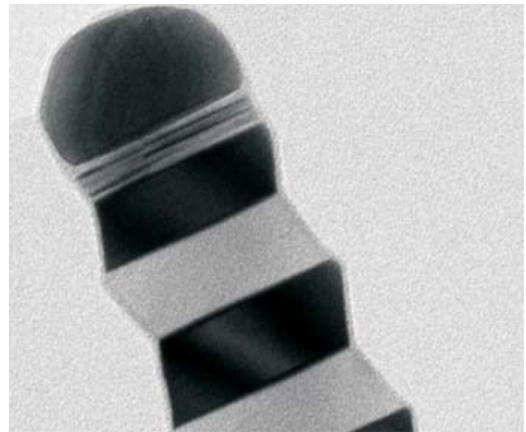
Fig 2. TEM image of the top part of an InP NW, closely below the Au catalyst particle, showing the highly regular twin superlattice structure.
