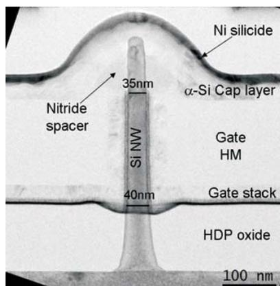
Fig 41. TEM cross-section of the final vertical 35nm NW TFET device (no top oxide isolation) with an advanced a-Si/TiN/HfO<sub>2</sub> gate stack
