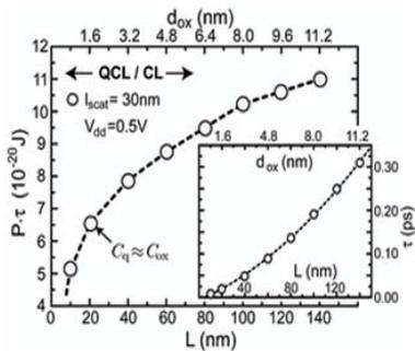
Fig 45. Power delay product and gate delay (inset) versus gate length and oxide thickness for conventional FETs as the transition from classical limit to the quantum capacitance limit is made.
