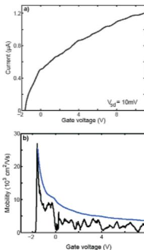
Fig 25. (a) pinch-off curve and (b) extracted field-effect (black) and effective mobilities (blue) of a high mobility core/shell nanowire.
