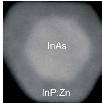
Fig 8. Dark-field TEM image of the InAs(core)/InP:Zn(shell) NW.
