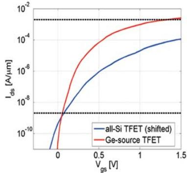
Fig 44. Comparison of  $I_{ds}$ - $V_{gs}$  characteristics of all-Si TFET (short gate) and the proposed heterostructure Ge-source Si-TFET, indicating the boost of the current with nearly 2 orders of magnitude to the same level as Si MOSFETs (dashed curves).
