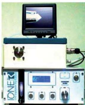
Fluid-electrodynamic device that generates an electrically charged nanoparticles or ions from a dispersion or solution.
