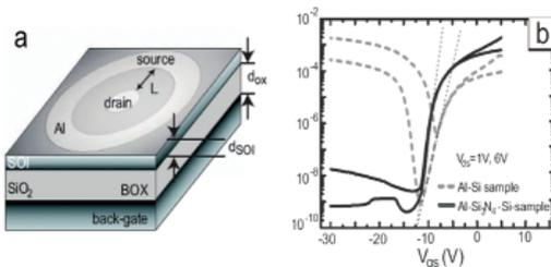
Fig 15. Schematic of a Schottky barrier pseudo-MOSFET and the corresponding transfer characteristics with and without an interface layer.
