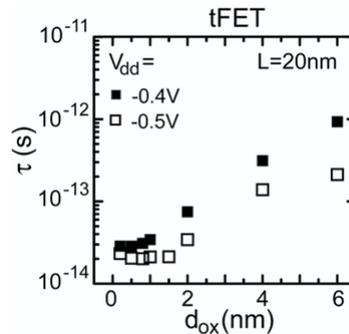
Fig 46. Gate delay versus oxide thickness for nanowire MOSFETs and tunnel FETs.
