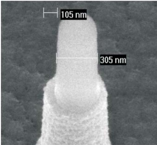
Fig 21. Vertical nanowire surrounded by a dielectric and a wrap gate.
