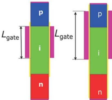
Fig 43. Schematic representation of the short-gate (left) and shifted-gate (right) concepts.
