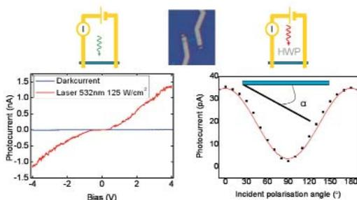
Fig 6. Photocurrent measurement on a single nanowire. Left: photocurrent as a function of applied bias. Right: photocurrent as a function of laser polarization.
