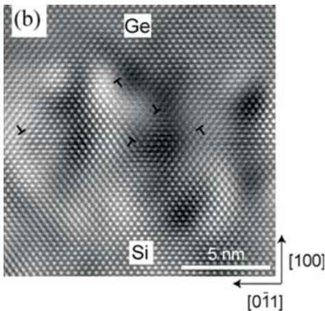
Fig 4. Cross-section TEM image of the Ge-Si interface.
