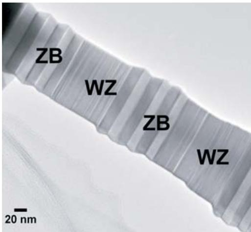
Fig 1. Polypotypic superlattice, with alternating zinc blende and wurtzite structure, along an InAs nanowire.
