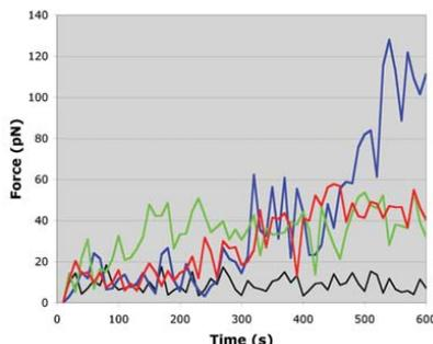
**Fig 2.** Cellular force measurements using nanowire arrays. (LEFT) Confocal fluorescence image of a growth cone on 40 nm diameter 5  $\mu\text{m}$  long nanowires. Scale bar 1  $\mu\text{m}$ . (RIGHT) Forces exerted on the nanowires highlighted in the left images. The forces range from 20 to 130 pN.
