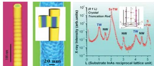
Fig 28. Longitudinal and radial heterostructures measured by Grazing Incidence X-ray Techniques and example of a truncation rod measurement showing the [111] stacking in a longitudinal InAs/InP heterostructure.
