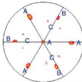
Fig 3. GaP wires next to a thick wire are taller than the second-nearest wires, which are taller than those in the middle of the field (furthest from the thick wire), showing that the growth rate of one wire is enhanced by the presence of another one and dependent on the catalytic alloy amount.
