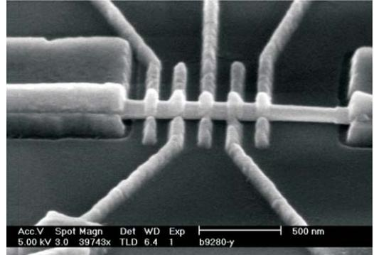
Fig 16. Horizontal InAs/InP nanowire with multiple gates.
