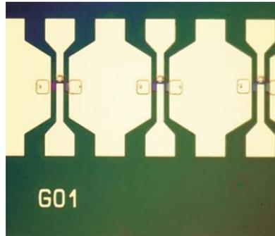
Fig 19. Top view of a fully processed RF-compatible vertical nanowire transistor structure.
