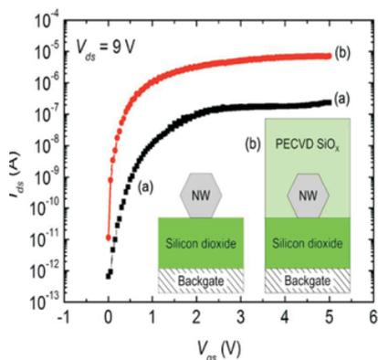
Fig 12. Transfer characteristic of a lateral nanowire n-MOSFET as fabricated surrounded by air (black) and encapsulated in SiO<sub>2</sub>.
