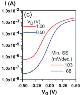
Fig 31. Sub-threshold I-V characteristics of an array of 55 vertical InAs nanowires.
