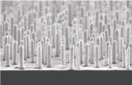
Fig 9. Si nanowires grown by use of an Al catalyst.
