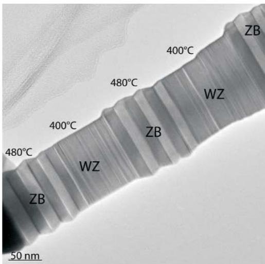
Fig 2. Transmission electron micrograph of a ZB-WZ polytypic superlattice in an InAs nanowire. The structure was achieved by periodically varying the growth temperature.
