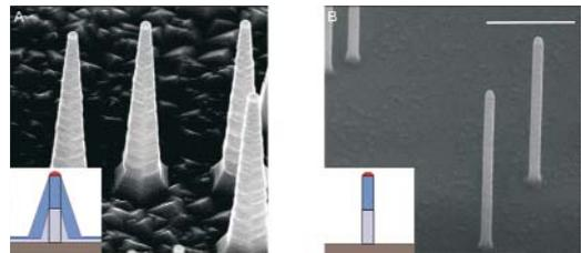
Fig 6. a) Tapered reference InP nanowires grown at a temperature of 450°C. b) Non tapered nanowires grown with HCl in the gas phase under otherwise identical growth conditions to a).
