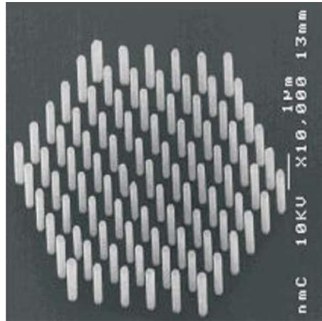
Fig 11. Epitaxial InAs nanowires grown on a Si(111) substrate from holes etched in a SiO<sub>2</sub> film.
