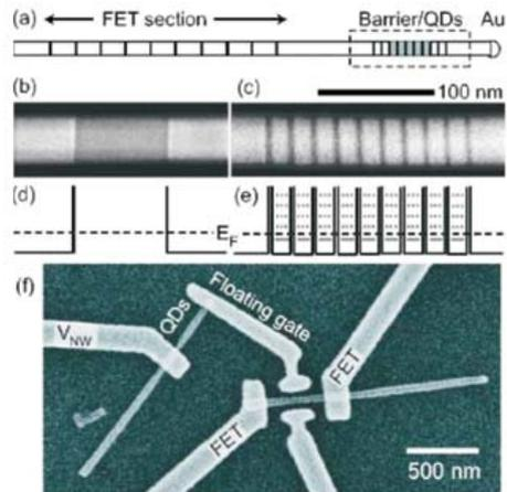
Fig 33. Design and implementation of a multiple quantum dot memory based on nanowires.
