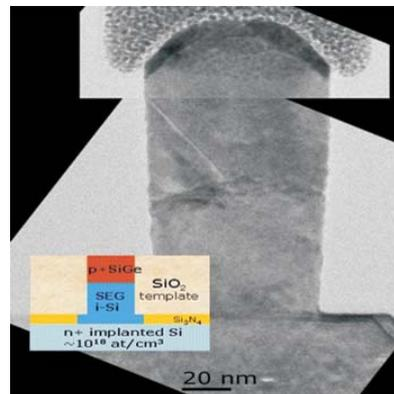
Fig 40. TEM micrograph of a 60nm wide Si/SiGe heterojunction nanowire.
