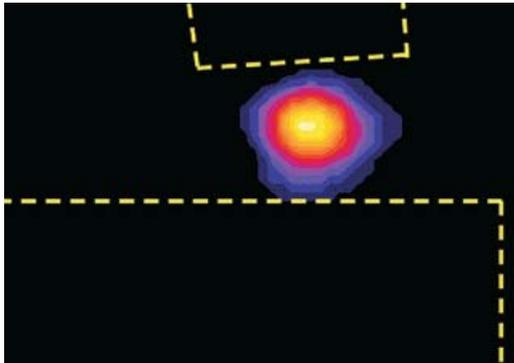
Fig 7. Optical microscope image of electroluminescent light coming from an InP NW LED, as collected by a CCD camera (the dashed lines show the positions of the electrodes).
