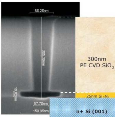
Fig 22. Cross-section of a via hole after plasma etch and hot phosphor opening of the Si<sub>3</sub>N<sub>4</sub> bottom layer.
