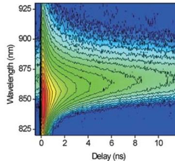
Fig 28. Spectrally and temporally resolved intensity map of the PL emission from  $\text{HfO}_2$  capped InP NWs.
