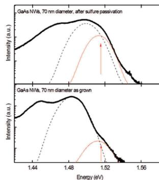
Fig 13. Photoluminescence spectrum of an as grown (bottom) and a passivated wire (top).
