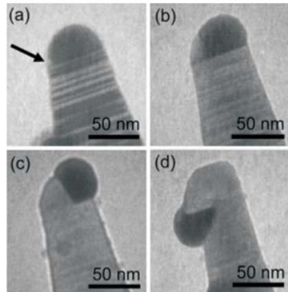
Fig 5. Images recorded during the growth of Ge on GaP nanowires by UHV-CVD.
