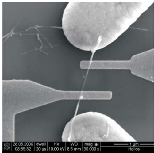
Fig 17. Si-nanowire FET with two gated Schottky contacts.
