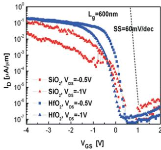
Fig 37. Transfer characteristics of silicon nanowire tunnel FETs with SiO<sub>2</sub> (red) and HfO<sub>2</sub> (blue) gate dielectrics.
