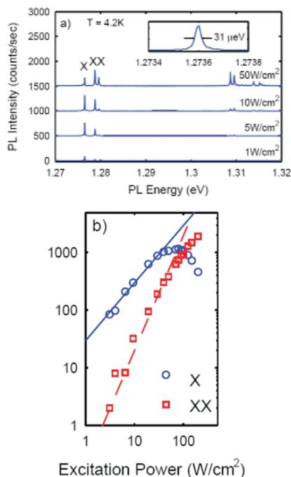
**Fig 3.** (a) Power dependence of the photoluminescence from a single quantum dot in a nanowire under continuous excitation at 532 nm. (b) Integrated power dependence of two narrow emission lines attributed to the exciton and biexciton. Samples grown by the Bakkers group.
