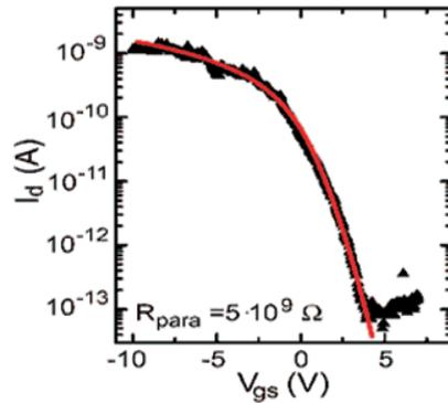
Fig 36. Transfer characteristics of a Si NW tunnel FET with top gate. The red line is calculated using the WKB approximation.
