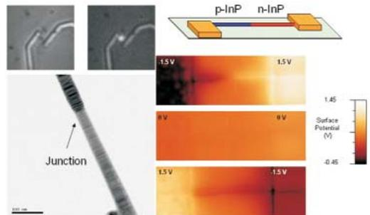
**Fig 5.** Single nanowire light emitting diode. Left: microscope image of the nanowire LED without and with forward bias. Bottom left: TEM image of a pn junction in an InP nanowire. Right: electrostatic force measurements under forward (top) and reverse (bottom) bias.
