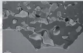
*Cross section through the front contact of a Si wafer-based solar cell. Taken with in-lens SE detector at 2 kV. Courtesy of Dr. F. Machalett, erSol Solar Energy AG, Erfurt, Germany.*
