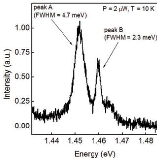
Fig 27. Micro photoluminescence spectrum showing emission from two InP nanowires with narrow linewidths of 4.7 meV and 2.3 meV, respectively.
