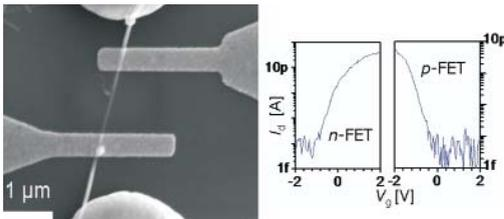
Fig 38. Silicon nanowire FET with two independent top gates, each coupling to a metal/semiconductor junction. The FET can be programmed as p- and n-type.
