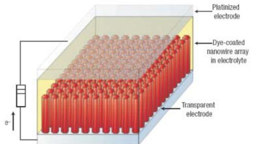
Schematic of a nanowire array for solar cell application.
