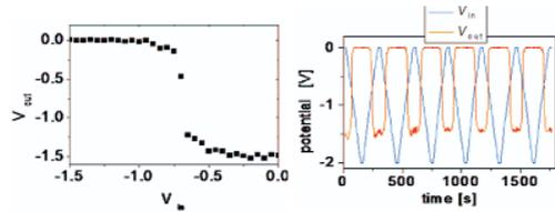
Fig 39. Silicon nanowire inverter characteristics; top: transfer characteristics, bottom: time resolved response.
