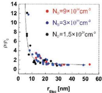
Fig 35. How the resistivity of silicon nanowires increases with decreasing diameter due to doping deactivation caused by a dielectric mismatch between the nanowire core and the surroundings.
