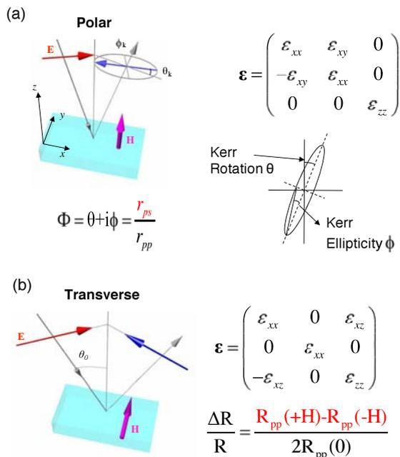
Figure 2. Scheme of the geometry and the relevant magnitudes for the two magneto-optical effects considered in this work: (a) polar Kerr configuration; (b) transverse Kerr configuration.
