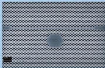
Photonic crystal with proximity effect correction
