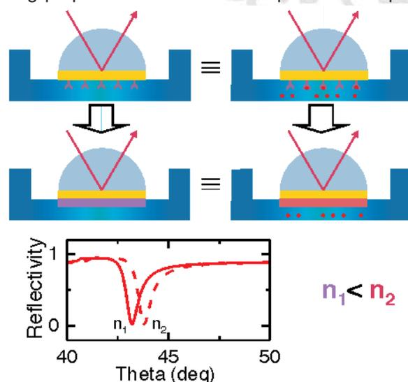
**Figure 1.** SPR schematic description in the Kretschmann configuration for plasmon excitation. The receptors can be seen as a layer of index  $n_1$  that upon recognition changes into  $n_2$ , causing a shift in the reflectivity curve.
