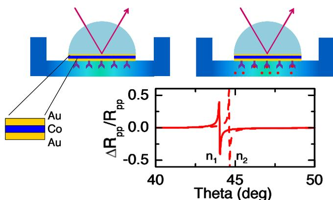
**Figure 3.** Transverse MO Kerr effect curve before and after a recognition process. The higher sensitivity comes from the higher slope when compared with conventional sensors.
