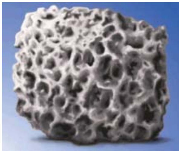
**Figure 4.** PLLA scaffold obtained by thermally induced phase separation
