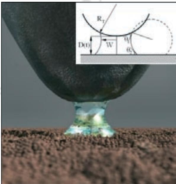
**Figure 1:** Artistic representation of a tip linked to a substrate through a water bridge. Inset: Schematic representation of the tip-neck-substrate system.
