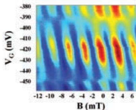
**Figure 1:** Interference pattern of the source-drain current in the ABI as a function of magnetic field  $B$  and gate voltage  $V_G$ . The red (blue) color corresponds to a maximum (minimum) intensity, i.e. to constructive (destructive) interferences between the electrons flowing in each of the ABI arms.
