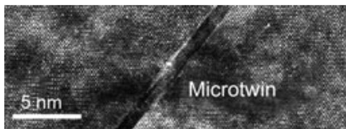
**Figure 1:** Surface of the FePt film (top): the microtwins can be seen (AFM image). These defects are organized in a quasi-periodic lattice that delimits the terraces. The color code indicates the relative height of the terraces (see vertical scale). TEM section of a microtwin (bottom).
