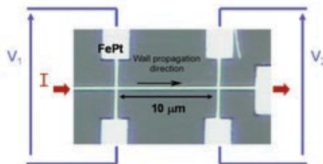
**Figure 3:** Overview of the nanostructure (optical microscopy). A current is injected in the central wire. By measuring the Hall voltage  $V_1$  and  $V_2$ , propagation of the domain wall through the first and the second cross is detected.
