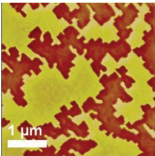
**Figure 2:** MFM image of the sample: two magnetic domains are observed (brown and yellow). The domain walls are trapped on microtwins.
