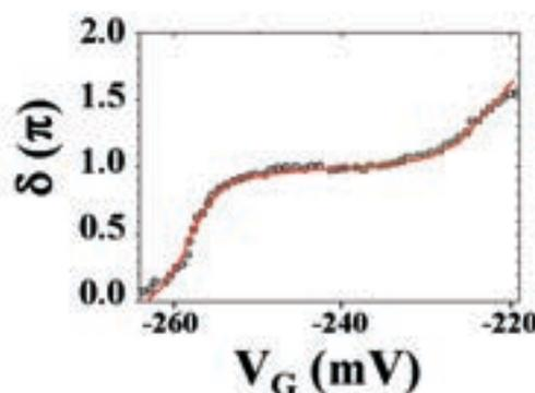
**Figure 2:** Comparison of theoretical and experimental results for the gate voltage ( $V_G$ ) dependence of the phase shift in the Kondo regime.
