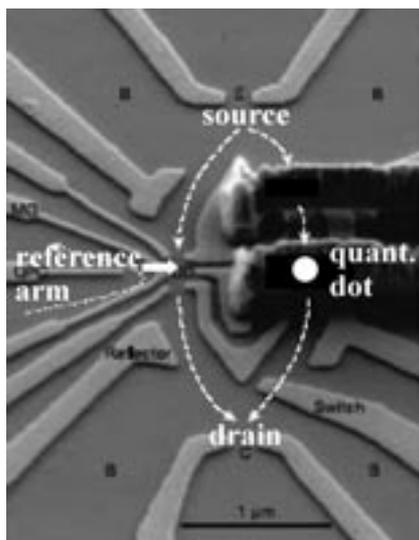
**Figure 3:** SEM picture of an Aharonov Bohm quantum interferometer. The two arms are depicted in white.
