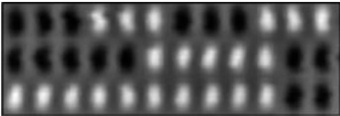
**Figure 2:** Magnetic imaging using the read head signal of a partially written area (white dots). The length of each information bit is 200 nm.
