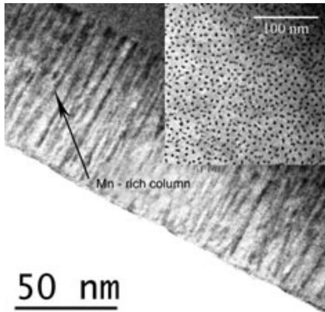
**Figure 1:** Plane view (inset) and cross-section in transmission electron microscopy of a GeMn layer. In the middle of the matrix, the self-assembled manganese-rich columns can be observed.
