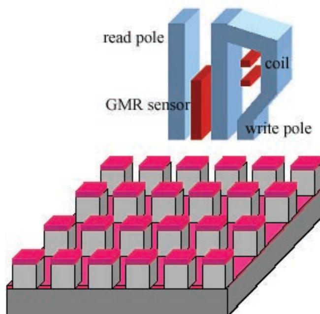
Figure 1: Layout of the magnetic read/write head and the discrete medium
