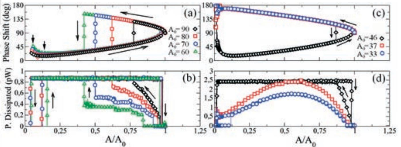
**Figure 3:** Phase (a) and power dissipated (b) vs normalized amplitude. The cantilever parameters are  $k=2N/m$ ,  $Q=100$ ,  $v=w_0 / (2\pi)=100kHz$ . (c,d) are the same as (a,b) but for lower amplitudes (and different cantilever constants:  $k=27.5N/m$ ,  $Q=400$ ,  $v=280kHz$ ). In the RR ( $\phi < 90^\circ$ ), the energy dissipated per oscillation is simply given by  $U_{dis}$ . The rest of simulation parameters can be found in reference [16]. (Based on Sahagún et al. [5]).
