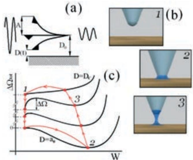
**Figure 2:** (a) Tip-cantilever-driver system. (b) Graphic representation of water neck formation/rupture. (c) Schematic representation of the formation/rupture process in tapping mode. (Based on Sahagún et al. [7]).
