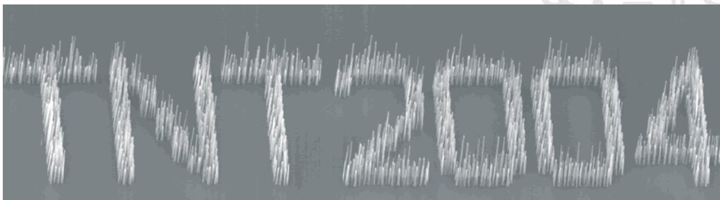
**Figure 2:** Carbon nanotubes ordered over a surface using electronic lithography techniques. The image shows the official logotype of the Trends in Nanotechnology conference (TNT2004) [8] (Courtesy of Ken Teo (Cambridge University (UK)))
