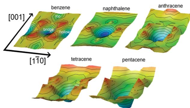
Fig. 2. Minimal potential energy surface maps of five polyacene molecules adsorbed on Cu(110) calculated with the ASSED+ code. The diffusion of polyacene molecule is more favorable in the [1-10] direction
