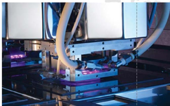
Ultraviolet light is generated directly inside the imprinting head by an array of 25 UV-LED Arrays.
