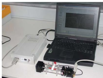
Fig. 1.6. Applications of NIL in optoelectronics for gas sensors. Schematics of a DBR laser diode. The DBR grating in this device concept is fabricated by using nanoimprint lithography. The DBR laser diode and its control electronics. (Nanoplus GmbH)
