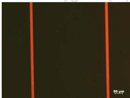
Figure 4.4: Waveguide imprinted in luminescent NC doped PMMA
