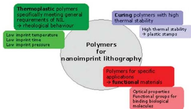
Figure 4.1: Approaches to polymers for nanoimprint lithography
