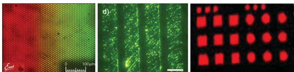
Fig. 2.3  $\mu$ CP of a double gradient of proteins for bio-chip applications, BSA-FITC in green, BSA-Cy3 in red (left image).  $\mu$ CP of stretched lambda-DNA complexed with a fluorescent conjugated polyelectrolyte (scale bar 15  $\mu$ m) (center image).  $\mu$ CP of oligonucleotides for bio-chip applications (right image). (images courtesy of CNRS-LPN, Linköping University, and CNRS-LAAS)
