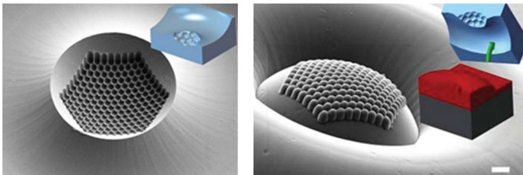
Fig. 1.3 Left: Towards 3D nanoimprinting. Fabrication of three-dimensional stamps by electro-beam lithography, focused ion beam and wet etching. Right: Structure of compound eyes fabricated by hot embossing on the thermoplastic polymer Zeonex. (M Tormen et al, TASC)
