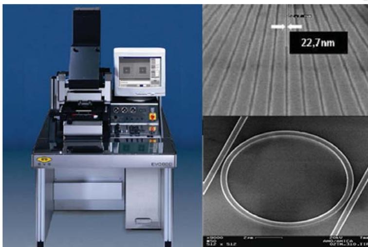
Fig. 2.1 EVG620 tool for soft UV molding (left). Imprinted high resolution pattern (upper right) and optical ring resonator structure (lower right). (Images courtesy of EV Group and AMO GmbH)
