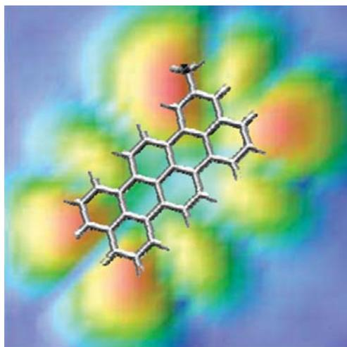
Fig. 3. ESQC-STM image calculation of a single methylterylene molecule adsorbed on two monolayers of NaCl(100) deposited on Cu(111) surface. The thin insulating film allows the decoupling of the electronic structure of the molecule from the metallic substrate. The structure of molecular orbitals can then be well resolved.
