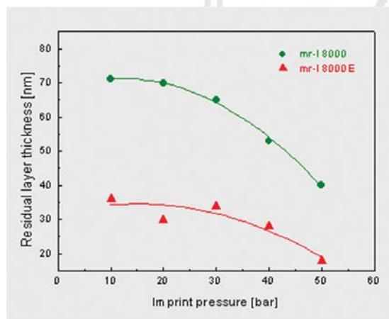
Figure 4.2: Residual layer thickness of new mr-I 8000E in comparison with "standard" mr-I 8000 as a function of imprint pressure, film thickness: 200 nm, Imprint: 10 s @ 160 °C, incomplete filling of stamp cavities
