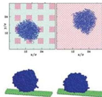
Fig. 6.3- The effect of surface patterning on droplet formation. Figure courtesy of Warsaw University of Technology and the Institute of Physics, Polish Academy of Science.
