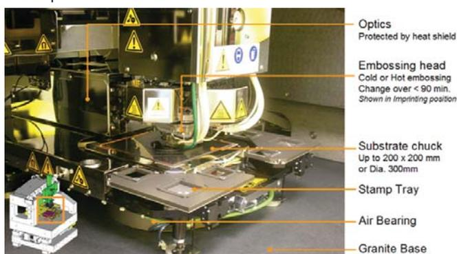
Parameters to control are: stamp-to-wafer leveling, alignment, force profile, temperature, UV-exposure and Material Dispense
