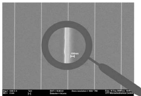
Fig. 1.7 Left: Roll-to-roll printing. Flexo unit tested using printing inks and polyaniline-toluene on paper. Right: SEM image of Ni stamp with 100 nm wide and 170 nm high ridges. (T Makela et al, VTT)
