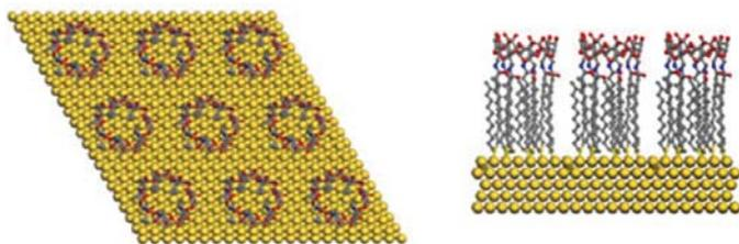
Fig. 6.4 - Plan and side-on views of a molecular printboard, a hexagonally-packed array of beta-cyclodextrin molecules anchored to gold using alkane-thioether chains. MD simulations provide atomic scale information on the stability and flexibility of such arrangements. Simulations performed at Tyndall National Institute in collaboration with the experimental work at Mesa+, University of Twente.
