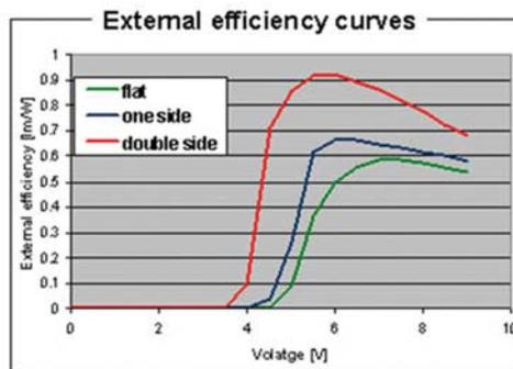
Fig. 1.5 Nanoimprint applications in organic opto-electronics. The NIL introduction in the light emitting technology allows the fabrication of high performance substrates on large area with a low cost process. A high increment of performances is obtained with double layer nanostructuring of the devices. (V Lambertini et al, CRF)
