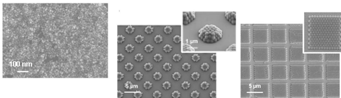
Fig. 2.4 Gold nanorods deposited by convective assembly (left image). Polystyrene particles (500 nm) assembled on an elastomer stamp and then printed on a gold coated silicon substrate (center and right image). (Images courtesy of CNR-IPCF and IBM Research GmbH)
