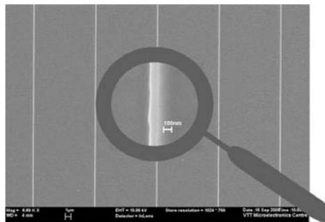
Fig. 1.7 Left: Roll-to-roll printing. Flexo unit tested using printing inks and polyaniline-toluene on paper. Right: SEM image of Ni stamp with 100 nm wide and 170 nm high ridges. (T Makela et al, VTT)
