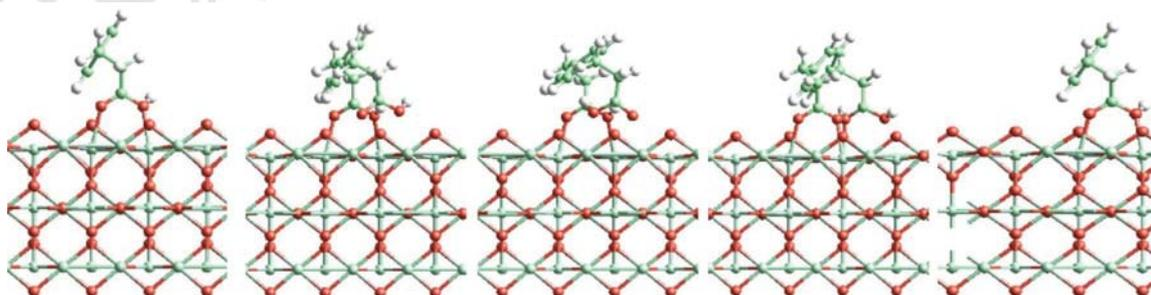
Figure 3: Illustration of a prototype 'walker' molecule on the  $\text{TiO}_2$  surface.
