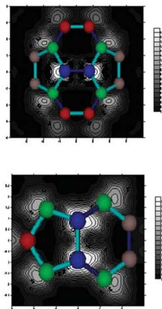
Fig. 2. Calculated AFM images of the C60 molecules adsorbed in two configurations on the Si(001) surface with either two hexagons or with a hexagon and a pentagon facing up the tip.
