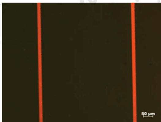
Figure 4.4: Waveguide imprinted in luminescent NC doped PMMA
