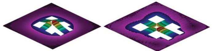
Fig. 6.2 – Side by side comparison of the stabilisation of MEMS membranes using corrugation rims. Left: Unstabilised, Right: Stabilised. Simulation work courtesy of Tyndall National Institute, performed in collaboration with fabrication of the membranes at EPFL.
