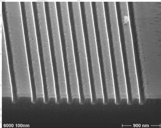
Figure 4.5 : mr-NIL 6000 test pattern, 100 nm trenches, 300 nm pitch, 200 nm film thickness
