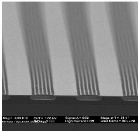
Fig. 1.2 Nanoimprinting for microfluidics. SEM micrographs of the processes samples with the new design. Long lanes of pores, ordered in groups of 3 or 5 rows, where imprinted. By dissolving the LOR (Lift-off-resist) below the pores, long channels are created which serve for fluid transport. (H Schiff et al, PSI)
