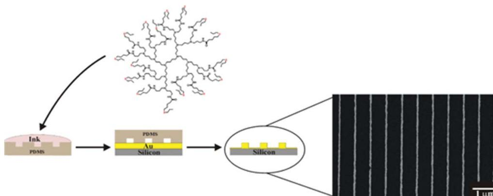
Fig. 2.2 100 nm wide lines produced by positive CP with dendrimer inks (image courtesy of University of Twente)
