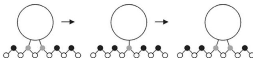
Fig. 3. Pivoting mechanism of C60 manipulation/diffusion on the Si(001) surface [5,7].
