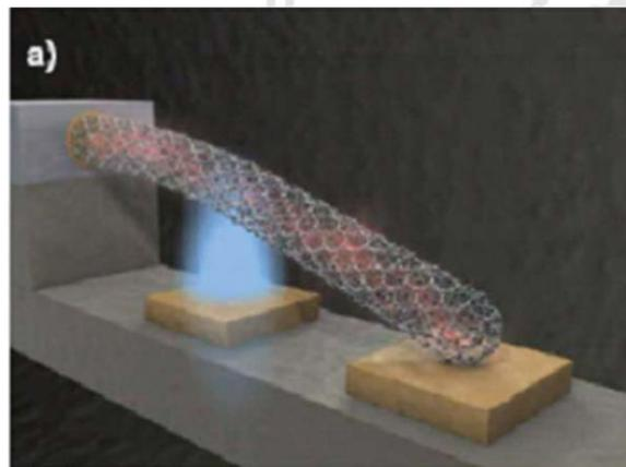
A singly-clamped conducting Carbon nanotube (diameter about 10 nm) is electrostatically bent by an electric field originating from the gate electrode to close the electric circuit between the source and drain electrodes.
