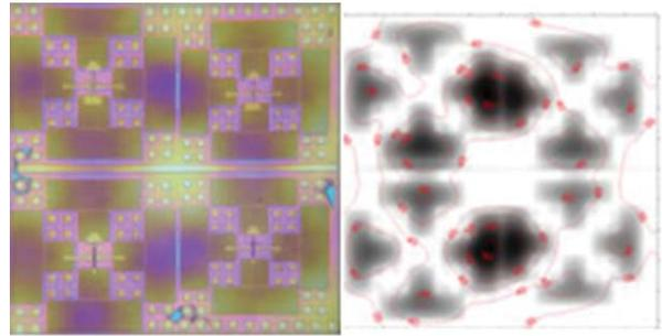
Fig. 6.1 – Coarse grain simulations of NIL patterned transfer compared to experiment. Left: Imprint (violet colour relates to thicker residual layer), Right: Results of modelling of pressure distribution in resist film and calculated distribution of elastic deformation of stamp in nanometres during imprinting. Simulation courtesy of Institute of Microelectronics Technology (IMT), Russian Academy of Science, experimental results courtesy of TASC-INFM.
