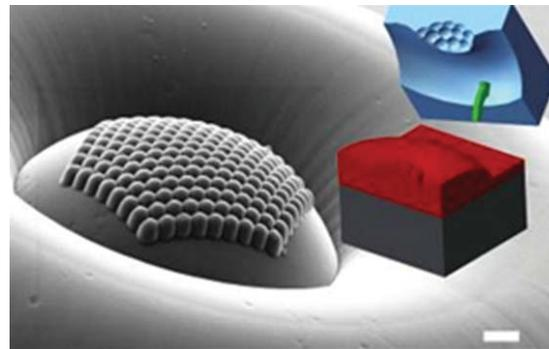
Fig. 1.3 Left: Towards 3D nanoimprinting. Fabrication of three-dimensional stamps by electro-beam lithography, focused ion beam and wet etching. Right: Structure of compound eyes fabricated by hot embossing on the thermoplastic polymer Zeonex. (M Tormen et al, TASC)
