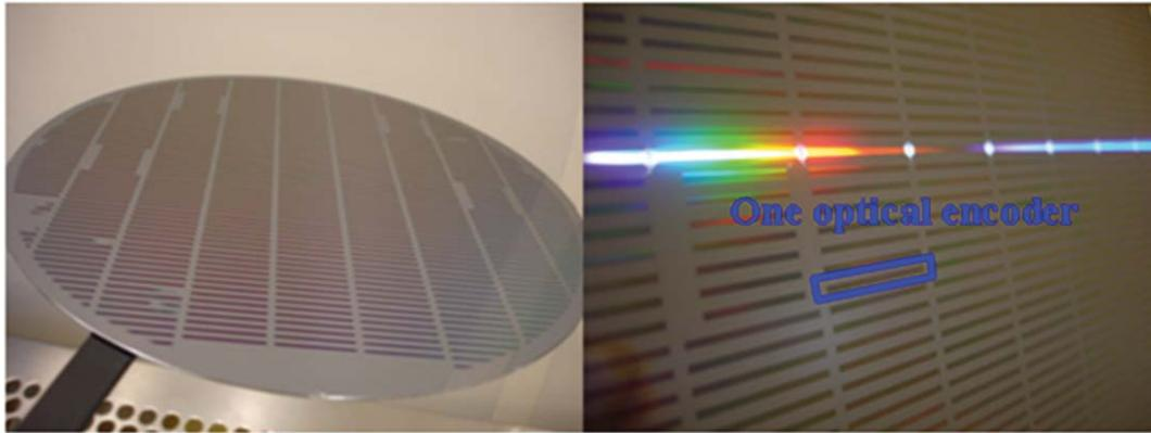
Fig. 1.1 Wafer-scale Nanoimprint lithography for optical applications. Full 200 mm silicon stamps and closer view of several optical encoders. Minimum feature size is 250 nm. (S Merino, Tekniker, and S Landis, LETI)
