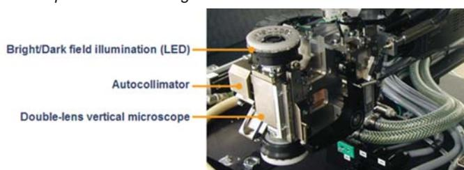
Stamp-to-Substrate alignment is performed using an Inter-Substrate Microscope which aligns features of the substrate to features of the stamp. The optics XY stage moves on air bearing to maintain the parallelism of the optical axis during displacement.
