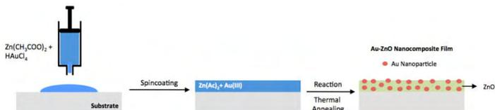
**Figure 1:** Procedure of the synthesis of Au-ZnO nanocomposite thin film.
