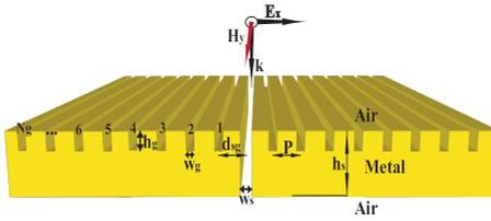
**Figure 1:** (Color). Schematic representation of the slit-groove array on a free-standing gold film of thickness  $h_s$ . The slit of width  $w_s$  is surrounded by  $2N_g$  grooves (width  $w_g$ , depth  $h_g$ , and period  $P$ ). The distance from the slit to the first groove,  $d_{sg}$ , is in principle different from  $P$ .
