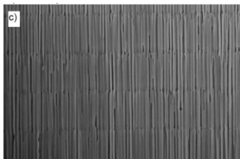
Figure 2: a) First three cycles of periodic anodization voltage used to produce an in-depth structured NAA with DBR structure and the corresponding current. b) reflectance spectra of the as-produced in-depth structured NAA and for the same structure after different pore widening times as indicated in the graph. c) FE-SEM cross-section picture of four cycles of the sample.
