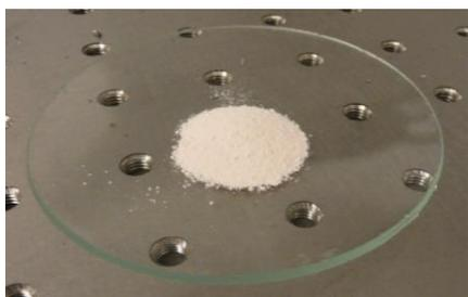
**Fig. 1:** Nanocrystals synthesized using the modified Pechini method.
