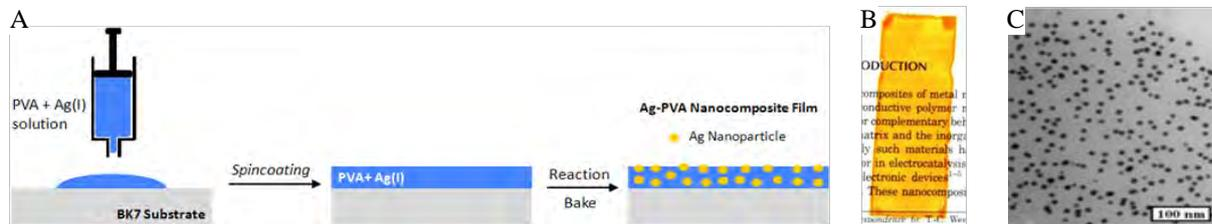
**Fig 1.** A) Schematic steps involved in the formation of Ag-PVA nanocomposite thin film; B) Image of the Ag-PVA film spincoated on soda-lime glass and C) TEM image..
