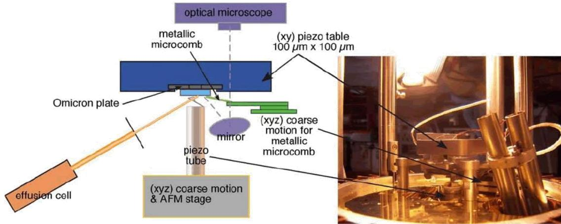
**Figure 2:** The micro cleanroom developed in the GNS group is based on a VT AFM/STM Omicron head which has been modified: the Omicron plate is now placed on a (XY) piezo table allowing fine motion on a (100 μm x 100 μm) area, an (XYZ) table allows the positioning of the microcomb, and the scene is seen through an optical microscope.
