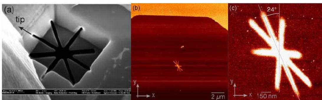
**Figure 5:** (a) SEM image of the cross drilled by FIB on one side of a cantilever tip ;(b) wide scale STM image ( $15 \mu\text{m} \times 15 \mu\text{m}$ ) obtained by moving the sample with the (XY) table; (c)  $1.5 \mu\text{m} \times 1.5 \mu\text{m}$  STM image showing the silver cross deposited.
