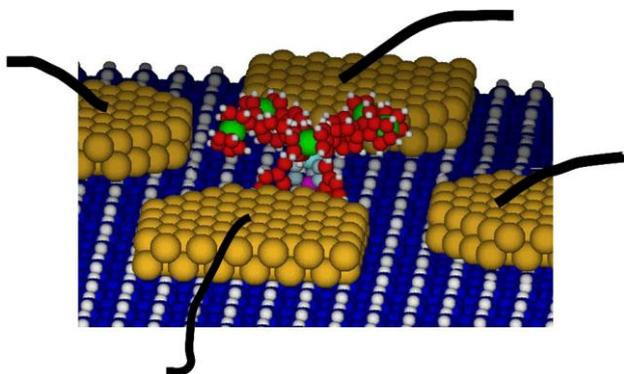
**Figure 1:** *A single molecule-motor [1] positioned between 4 Au nano pads constructed on the Si(100)-H surface. The motor is driven by the tunnelling electrons sequentially transferred through the motor wings. The 4 black wires getting out of the surface are indicative of the interconnections strategy to be developed.*
