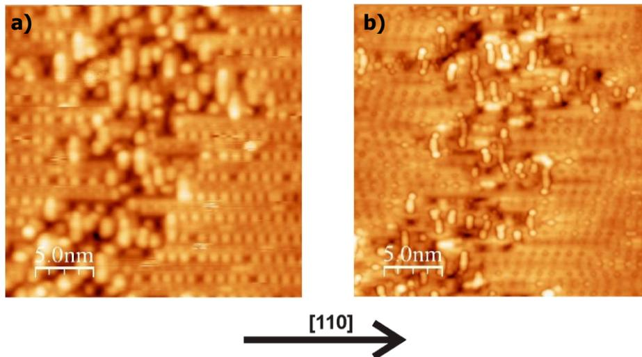
**Figure 3:** InSb(001) surface distorted during gold deposition. The sample was relatively quickly cooled down after evaporation process was ended. (a) bias voltage:  $2V$ , tunnelling current:  $100pA$ ; (b) bias voltage:  $-0.5V$ , tunnelling current:  $100pA$ .
