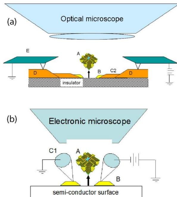
**Figure 2:** Scheme of the atomic scale interconnection machines for (a) wide and (b) moderate surface band gap substrates. A: Atomic scale circuitry, B: Contacting metallic nanopads, C1: Ultrasharp metallic tips, C2: Nanowires, D: Microelectrodes, E: Metallic microcantilevers
