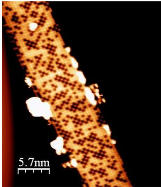
**Figure 2:** High resolution image of  $AuIn_2$  alloy nanowire; bias voltage:  $-2V$ , tunnelling current:  $5pA$ .
