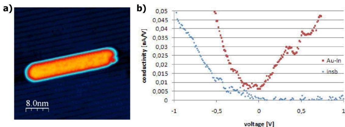
**Figure 1:** (a) High resolution STM image of gold nanowire formed on InSb(001) surface. Bias voltage:  $-0.5V$ , tunnelling current:  $25pA$ . (b) Conductance as a function of bias voltage for gold alloy nanowire (red dots) and InSb substrate (blue dots)
