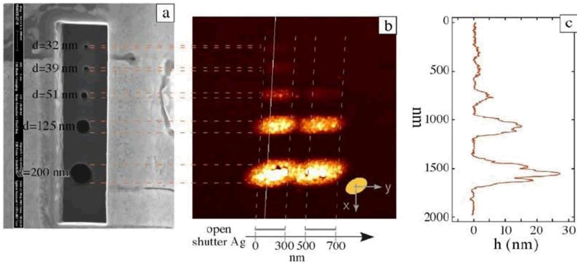
**Figure 6:** (a) 5 holes of increasing diameter drilled on a cantilever tip; (b) AFM image after deposition of silver ( $48 \text{ \AA}/\text{mn}$ ) while moving the substrate at  $20 \text{ nm}/\text{mn}$ ; (c) cross section along the white line.
