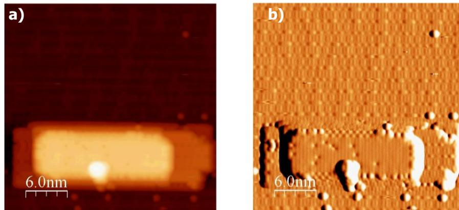
**Figure 4:** STM scans showing gold alloy nanowire with surrounding substrate surface reconstructed via post-deposition annealing. Bias voltage: -2V, tunnelling current: 100pA. (a) topographic image; (b) error signal.
