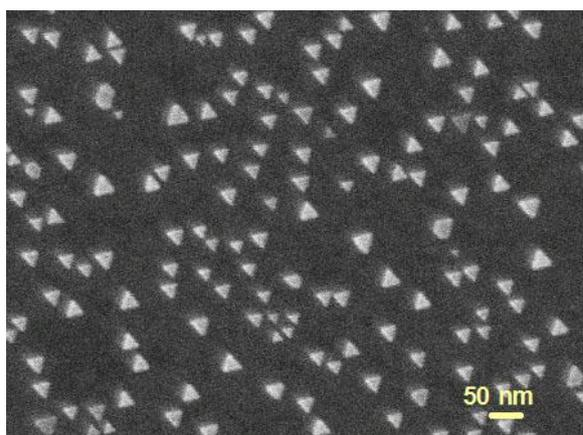
**Figure 2:** SEM image of the distribution of Au nano-islands on  $\text{MoS}_2$  after the fabrication process detailed in section 4.4. Many nano-islands are 30 nm in lateral size. Notice also the very sharp end at each summit of these triangles.
