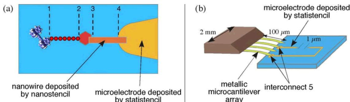
**Figure 1:** In the GNS group of Toulouse, the interconnects 3 and 4 are made by nanostencil with the micro cleanroom (a), and the interconnect 5 consists of a metallic microcantilever array contacting pads at the end of microelectrodes deposited by the static stencil process.
