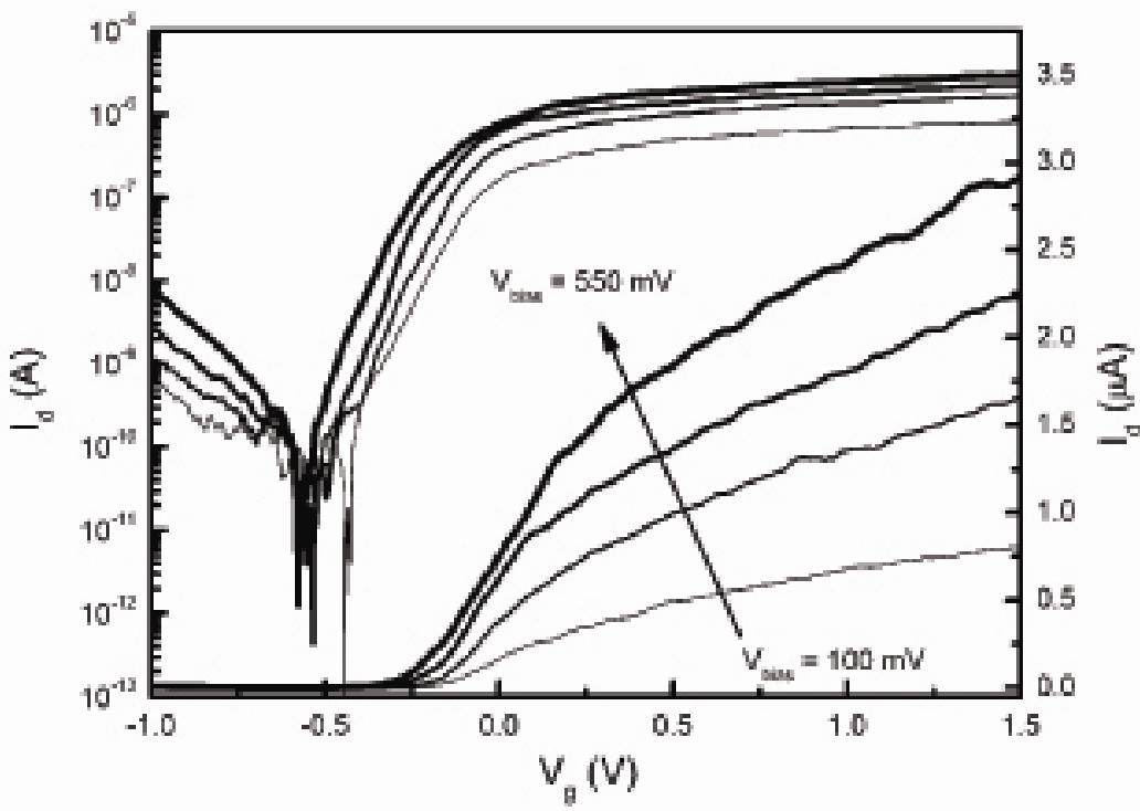
**Sub-threshold swing smaller than 60mV @ RT and threshold voltage**
