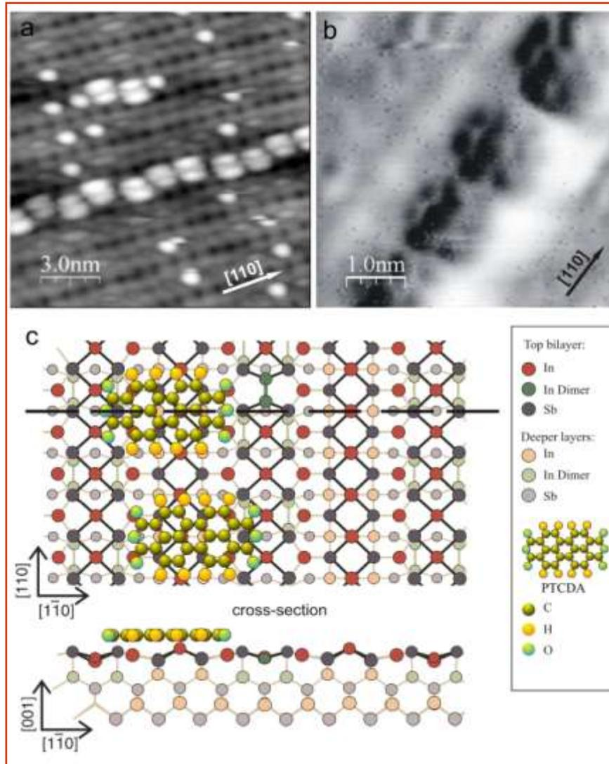
*PTCDA molecules assembled on reconstructed InSb (001) surface. a) Topography map of occupied states taken at 77 K and the sample bias of -1.0 V; b) Tunneling current map taken at 77 K and the sample bias of -0.75 V; c) “ $\zeta$ -model” of the  $c(8 \times 2)$  InSb (001) surface with a schematic model illustrating possible adsorption sites of PTCDA molecules.*
