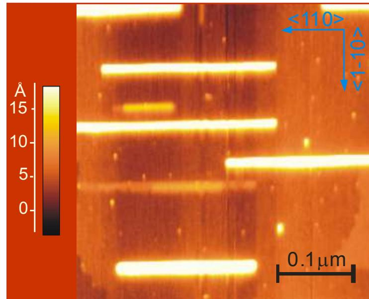
**Local CPD mapping allows for following conclusions: -low height wires (1-2 layers) have the same chemical nature as the substrate, higher wires have CPD clearly different from the substrate corresponding to large Au islands.**
