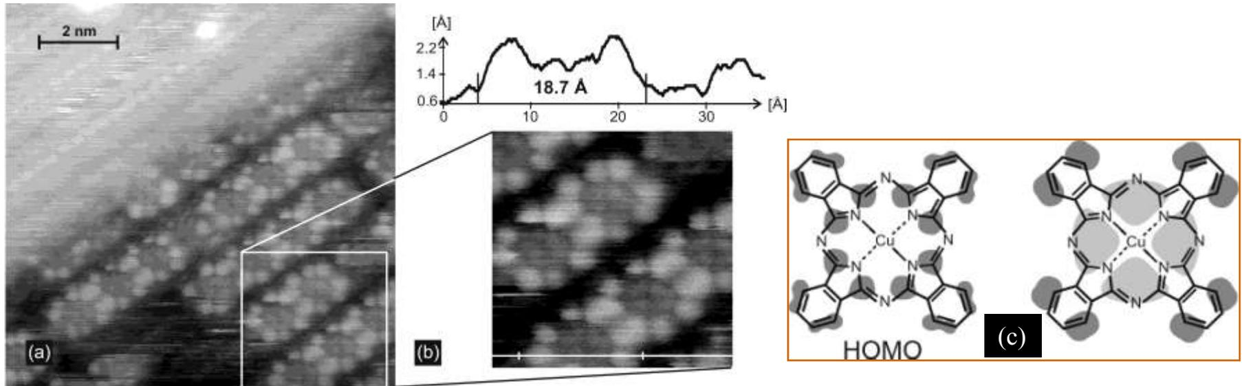
(a). STM image size: 15 nm  $\times$  15 nm, sample bias: -1 V, tunneling current: 0.6 nA. (b) Cross section along the long axis of the CuPc molecule (white solid line) indicating an additional fourfold structure in the STM contrast. (c) Schematic comparison of the experimental STM contrast recorded at negative sample bias (-1 V) with the DFT calculations of Lee for HOMO
