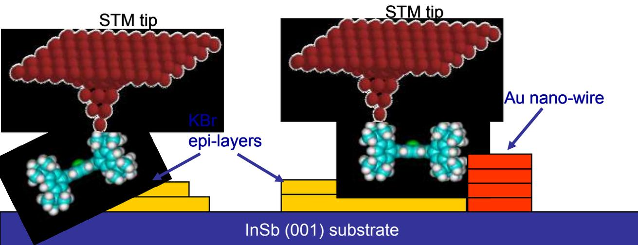
The molecule is assembled either across a nano-island step edge (insulator/semiconductor), or upon an insulator layer attached to a conductive nanowire. STM tip acts as a probe electrode; a role of the second electrode is taken by the conductive substrate.
