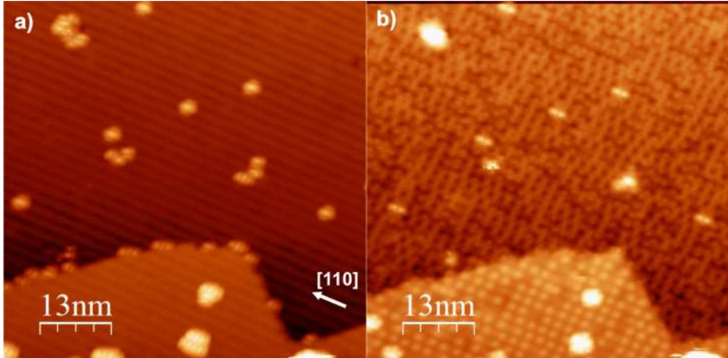
**A pair of 63x63 nm<sup>2</sup> STM images showing the same area taken with a) U=-2,3V, I=6pA; b) U=2,3V, I=6pA. The region in the upper part of the images is covered by a monolayer of KBr, while in the lower part an edge and a small fragment of a second-layer island is visible. Protrusions in filled state image a) are PTCDA molecules.**
