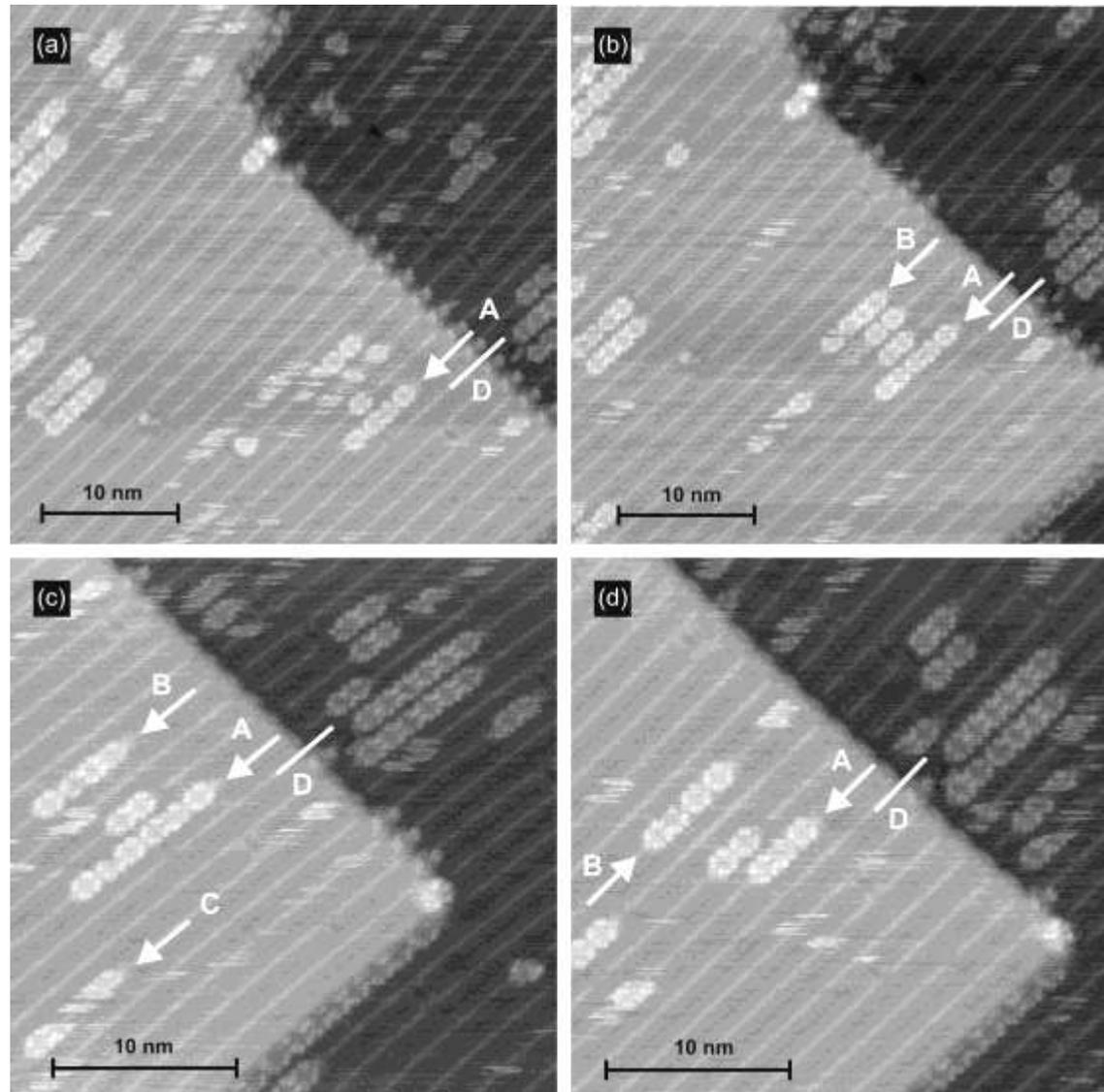
Demonstration of the tip-induced modification and the detail of decorated step edges. (a) 40 nm x 40 nm, -1 V, 0.3 nA. (b) 40 nm x 40 nm, -1 V, 0.15 nA. (c) and (d) 30 nm x 30 nm, -1 V, 0.15 nA.
