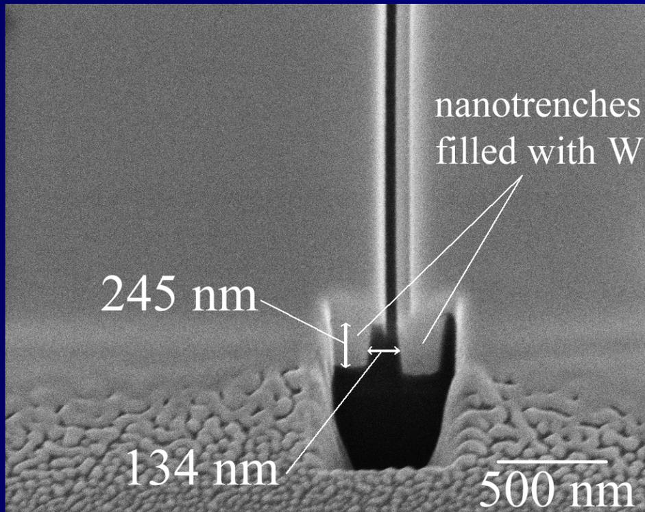
Viewing at  $52^\circ$  by *in situ* cross section and e<sup>-</sup> imaging
