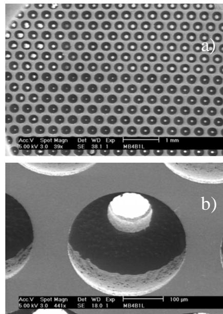
Fig. 3 SEM pictures of a silicon aperture plate. a) hexagonal array of 300  $\mu\text{m}$  diameter lens apertures at 400  $\mu\text{m}$  pitch and current limiting apertures ranging from 30-90  $\mu\text{m}$  in diameter. b) Close up of a lens hole with the current limiting aperture directly behind it.
