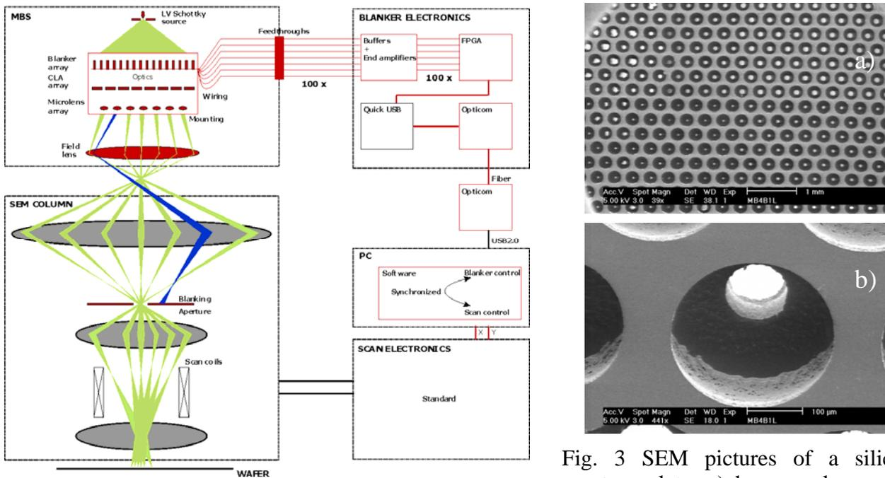
Fig. 2 Schematic overview of the Multi-beam SEM indicating the MBS unit, SEM column and the hardware necessary for synchronizing scanning and blanking.
