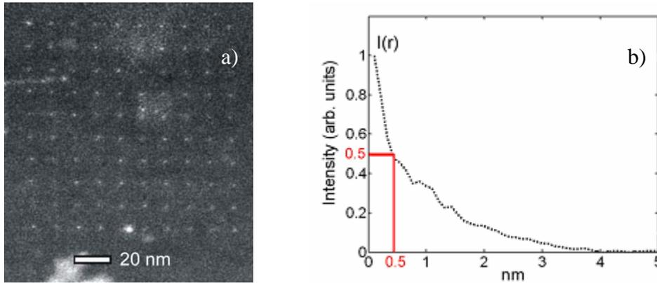
Fig. 1. a) a 10 by 10 array of dots, deposited from  $W(CO)_6$ . b): average radial intensity profile, showing a full width at half maximum of 1.0 nm.
