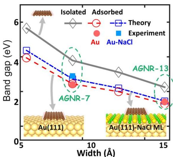
**Figure 1:** Quasiparticle band gap of the isolated and substrate-supported armchair graphene nanoribbons (AGNRs) as a function of their width. Energy levels in the substrate supported AGNRs are strongly renormalized by the substrate induced screening effect resulting in the reduction of the band gap.
