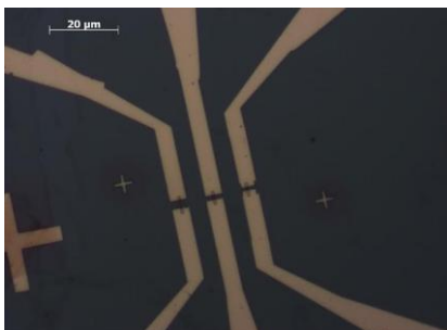
Figure 2: Suspended graphene resonators protected with HSQ in between gold electrodes.
