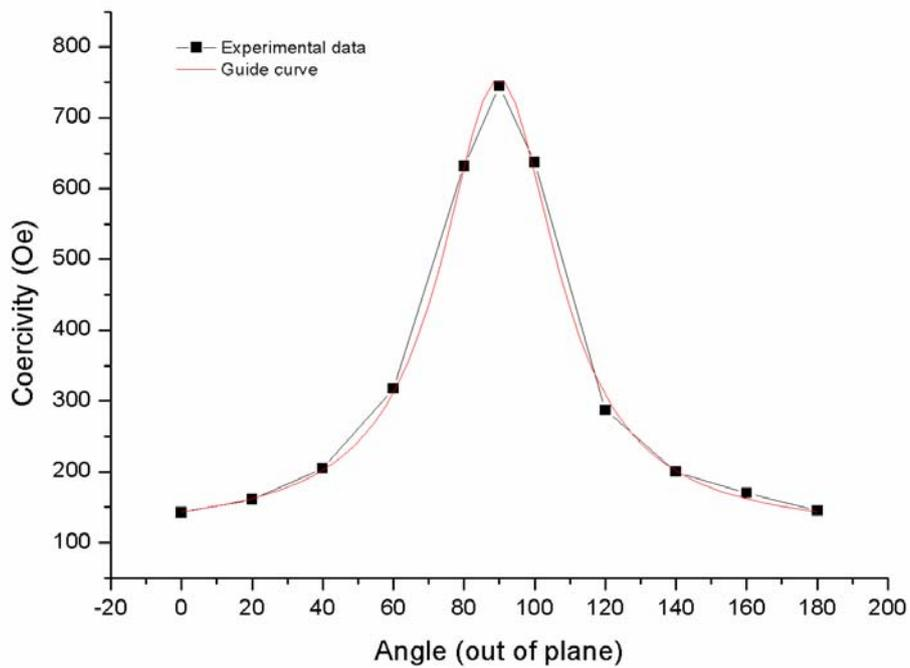
Fig 2 – Coercivity as function of the out of plane angle.
