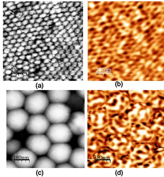
Figure 1: (a) AFM and (b) MFM image of the sample with a lattice parameter of 105nm. The Co thin film thickness is Co 30 nm. (c) AFM and (d) MFM image of the sample with a lattice parameter of 180nm. The Co thin film thickness is Co 30 nm.
