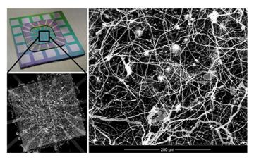
Fig. 1 > A look inside the ASN device reveals its highly interconnected architecture which comprises synaptic circuit elements at each point of contact between nanowires. The collective interactions between these atomic switches result in unique, emergent properties which have shown significant potential for neuromorphic computing./
