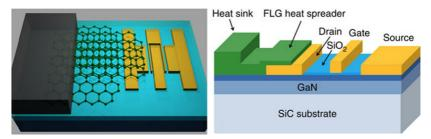
Fig. 4 > (Left) Schematic of the FLG-graphite heat spreaders attached to the drain contact of the AlGaN/GaN HFET. (Right) Device structure schematics showing the graphene-graphite quilt used in the simulation for the heat spreader optimization. Dark blue indicates the AlGaN barrier layer [1]./
