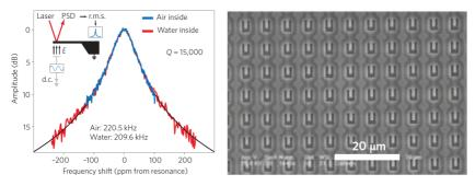
Fig. 10 > (Left) Resonance spectrum of a single mechanical resonator. The quality factor of the device is unaffected when the channel is filled with water (red line). (Right) Array of silicon cantilevers [5]./
