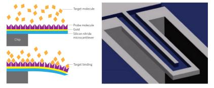
Fig. 9 > [5] (Left) Schematic of static-mode surface-stress sensing MEMS device. (Right) Suspended microchannel resonator (SMR). The fluid containing the target molecules flows through a channel inside the device and binds to the inner flow-channel walls, while the resonator oscillates in air or vacuum./
