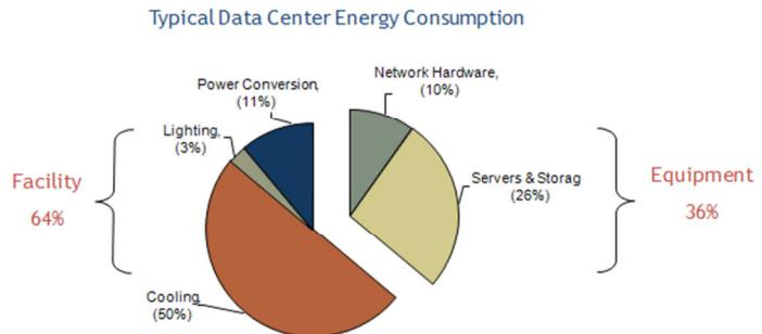
**Fig. 5** Typical distribution of the energy consumption in a data centre [23].
