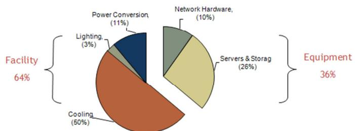
Fig. 5 > Typical distribution of the energy consumption in a data centre [23].
