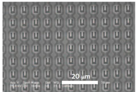
**Fig. 10 >** (Left) Resonance spectrum of a single mechanical resonator. The quality factor of the device is unaffected when the channel is filled with water (red line). (Right) Array of silicon cantilevers [6].
