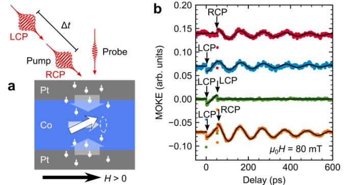
**Figure 1.** **a** Schematic representation of the double pump excitation scheme and spin excitation in Pt to drive FMR dynamics in the FM layer. **b** TR-MOKE measurements of OSOT-driven FMR dynamics and demonstration of coherent control.
