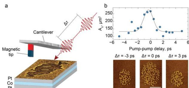
**Figure 1. Dual-pulse excitation and MFM probing of Pt/Co/Pt.** a) Schematics of the experimental setup of dual-pulse excitation and MFM probing. b) Switched area as a function of pump-pump delay. The lower panel shows MFM images of the nucleated patterns after dual-pulse excitation. The scale bar is  $20 \mu\text{m}$ .
