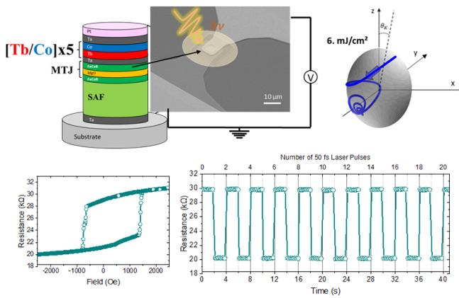
**Figure 2.** Illustration of the all-optical writing and electrical reading of an AOS MTJ stack showing SEM image of a 100-nm diameter pillar. Out of plane field hysteresis loop and resistance measurement after application of laser-pulse demonstrating toggle switching.
