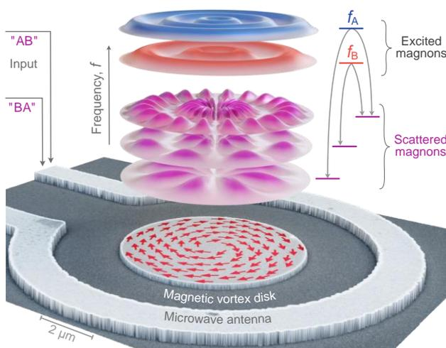
**Figure 1.** Working principle of a magnon-scattering reservoir. Radiofrequency pulses with different temporal order but the same average frequency content are used to trigger nonlinear scattering between the magnon eigenmodes in a magnetic vortex disk. The dynamic response is experimentally detected using Brillouin-light-scattering microscopy. In contrast to a linear system, the magnon-scattering reservoir produces different outputs depending on the temporal order of the input.
