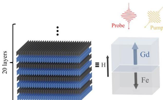
**Figure 1.** Schematic picture of studied Gd/FeCo multilayered structure.
