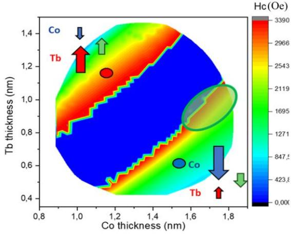
**Figure 1.** Multilayer thickness of  $[Tb/Co]_5$  showing helicity independent switching in cobalt rich highlighted green region under  $3.8\text{mJ}/\text{cm}^2$  50fs laser pulse.
