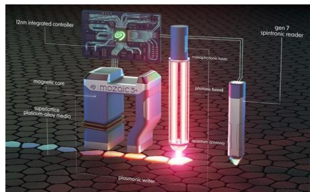
**Figure 1.** Critical Technology Innovations enabling Seagate's MOZIC3+ HAMR Product platform.
