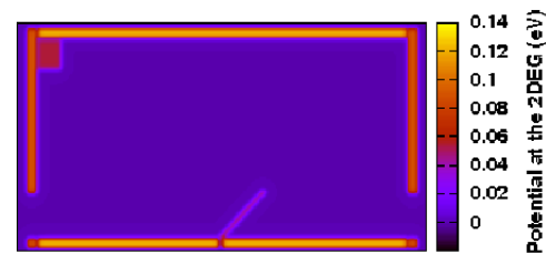
Fig. 3. Potential landscape at the 2DEG level for a mesoscopic cavity with a depletion gate at the upper left corner and a deflector gate in the middle of the bottom boundary of the cavity.
