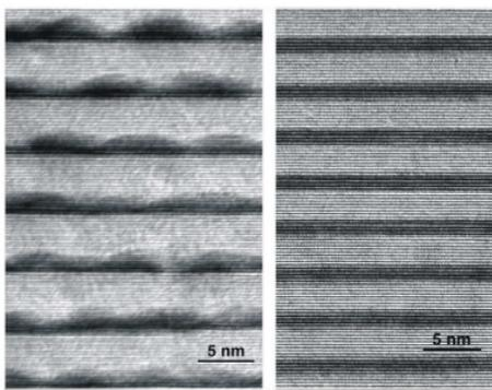
Fig. 1. High-resolution TEM images of (0001)-oriented GaN/AlN QD (left) and QW (right) superlattices.
