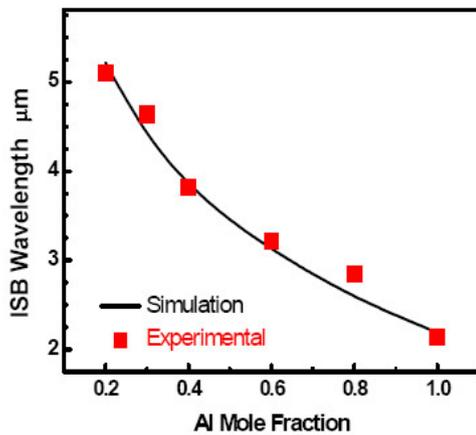
Fig 3. Variation of ISB transition energy with Al mole fraction on the barrier
