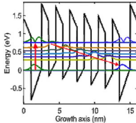
Fig 2. Band diagram and energy levels in one stage of the structure. (Red arrow) direction of electron relaxation (Bold lines) denote states involved in optical transitions.
