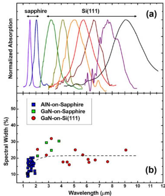
Fig 4 (a). IR absorption spectra for TM-polarized light measured in GaN/Al(GaN) superlattices grown either on sapphire or on Si(111) templates. (b) spectral width of the samples absorbing from NIR to MIR range.
