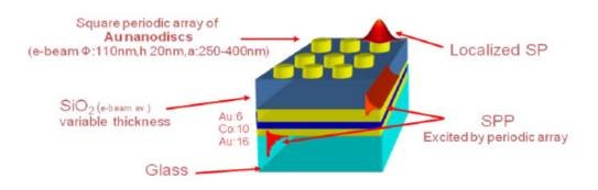
Figure 1. Configuration sustaining LSP, SPP and magneto-optical activity analyzed in this work.
