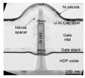
Figure 43. TEM cross-section of the final vertical 35nm NW TFET device (no top oxide isolation) with an advanced a-Si/TiN/HfO<sub>2</sub> gate stack
