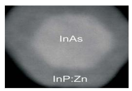
Figure 8. Dark-field TEM image of the InAs(core)/InP:Zn (shell) NW.
