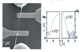
Figure 40. Silicon nanowire FET with two independent top gates, each coupling to a metal/semiconductor junction. The FET can be programmed as p- and n- type.
