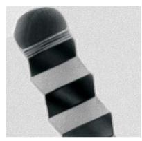
Figure 2. TEM image of the top part of an InP NW, closely below the Au catalyst particle, showing the highly regular twin superlattice structure.
