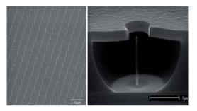
Figure 3. (a) Array of MWCNTs of height 5 μm and separation 5 μm[28] (b) Individual MWCNT grown in a micropore etched into SiO2 using a self alignment method [33].
