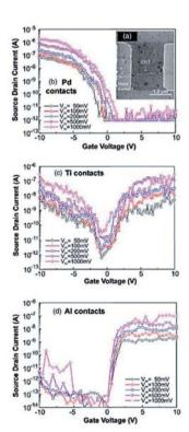
Figure 13. SWNT-FET transistor characteristics with different contacts. Top, Pd makes and ohmic contact which results in p-type conduction. Centre, Ti contacts result in strong ambipolar behaviour. Bottom, Al makes a Schottky contact which results in n-type conduction but with a strong leakage current.
