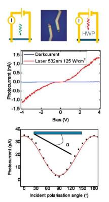
Figure 6. Photocurrent measurement on a single nanowire. Left: photocurrent as a function of applied bias. Right: photocurrent as a function of laser polarization.
