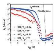
Figure 39. Transfer characteristics of silicon nanowire tunnel FETs with SiO<sub>2</sub> (red) and HfO<sub>2</sub> (blue) gate dielectrics.
