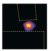
Figure 7. Optical microscope image of electroluminescent light coming from an InP NW LED, as collected by a CCD camera (the dashed lines show the positions of the electrodes).
