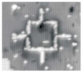
Figure 3. Ultra-high-vacuum STM image of a substrate after the fabrication with single-atom manipulation, of a complete interconnection circuit for an OR gate, obtained by removing hydrogen atoms from a silicon hydride surface.
