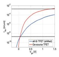
Figure 46. Comparison of  $I_{ds}$ – $V_{gs}$  characteristics of all-Si TFET (short gate) and the proposed heterostructure Ge-source Si-TFET, indicating the boost of the current with nearly 2 orders of magnitude to the same level as Si MOSFETs (dashed curves).
