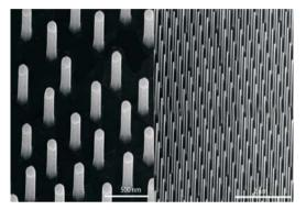
Figure 1. Scanning electron micrographs of gold particle-assisted, MOVPE grown, InAs nanowires in regular arrays, where the positions of the gold particles have been defined by electron beam lithography.
