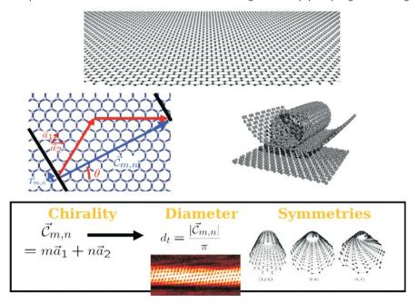
Figure 5. A carbon nanotube consists of a rolled up sheet of graphene.
