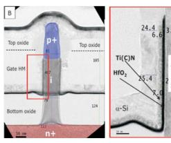
Figure 18. Cross section of the vertical TFET featuring 3nm HfO<sub>2</sub>, 7nm TiN and 25nm a-Si gate stack around the nanowires.
