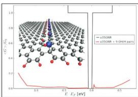
Figure 6. Functionalization of graphene nanoribbons.
