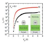
Figure 12. Transfer characteristic of a lateral nanowire n-MOSFET as fabricated surrounded by air (black) and encapsulated in SiO<sub>2</sub>.
