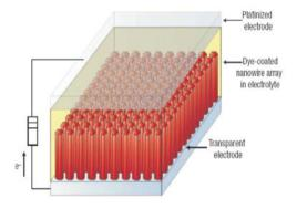
Figure 1. Schematic of a nanowire array for solar cell application.
