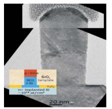
Figure 42. TEM micrograph of a 60nm wide Si/SiGe heterojunction nanowire.
