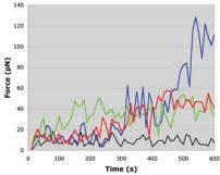
Figure 2. Cellular force measurements using nanowire arrays. (LEFT) Confocal fluorescence image of a growth cone on 40 nm diameter 5  $\mu$ m long nanowires. Scale bar 1  $\mu$ m. (RIGHT) Forces exerted on the nanowires highlighted in the left images. The forces range from 20 to 130 pN.
