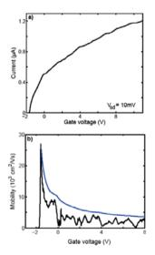
Figure 25. (a) pinch-off curve and (b) extracted field-effect (black) and effective mobilities (blue) of a high mobility core/shell nanowire.
