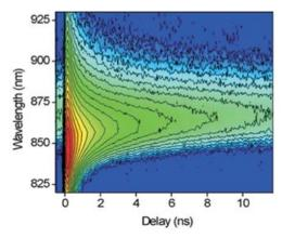
Figure 28. Spectrally and temporally resolved intensity map of the PL emission from  $HfO_2$  capped InP NWs.
