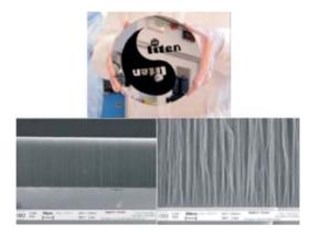
Figure 5. Dense forest of Small diameter MWCNT from left to right: a) Patterned layer on a 200mm layer b) 50μm high forest on conductive layer of TiN c) close view of the material with individual CNT making bundles of 60nm of diameter (courtesy of CEA-LITEN).
