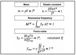
Table 1. Table summarizing how the properties of a mechanical system scale down with the reduction of its dimensions [10].
