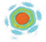
Figure 30. Coherent diffraction of single 95 nm Si nanowire (111) Bragg reflection. The "ab initio" analysis of this pattern allows reconstructing the shape of the NW.
