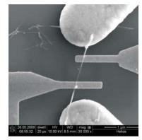
Figure 17. Si-nanowire FET with two gated Schottky contacts.
