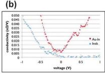
Figure 3. Exploring the surface science of interconnects: fabrication of Au nanowires on the InSb(001) surface in the UHV to be interconnected on a Fig. 2D UHV interconnection machine.(a) High resolution STM image of Au alloy nanowire formed on InSb(001) surface by a good selection of the surface annealing temperature. Bias voltage: -0.5V, tunnelling current: 25pA. (b) STS conductance measured using an
