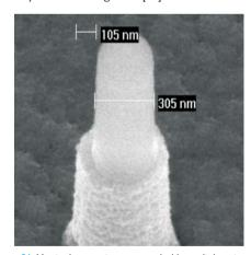
Figure 21. Vertical nanowire surrounded by a dielectric and a wrap gate.
