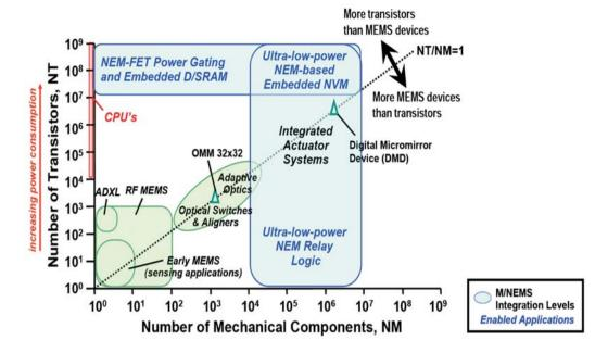
Figure 2. Summary of state of the art and future devices as a function of the number of transistors (NT) and the number of mechanical components (NM). Source: ITRS whitepaper authored by A. Ionescu (EPFL) et al.
