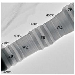
Figure 2. Transmission electron micrograph of a ZB-WZ polytypic superlattice in an InAs nanowire. The structure was achieved by periodically varying the growth temperature.
