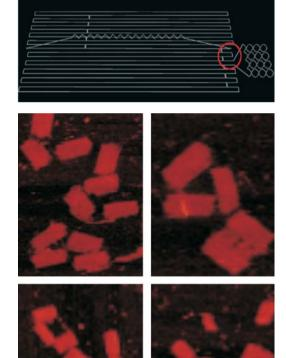
Figure 4. Assembly of bridged DNA origamis, a DNA single strand is kept unpaired to curve and bridge DNA origamis. Above scheme of the calculated structure. (courtesy JM Arbona, J. Elezgaray, JP Aimé.
