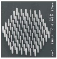
Figure 11. Epitaxial InAs nanowires grown on a Si(111) substrate from holes etched in a  $SiO_2$  film.
