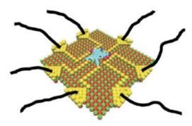
Figure 1. A possible surface implantation of a molecule logic gate. The presented molecule fi adder was designed following a Quantum Hamiltonian Computer approach [9]. The interconnection architecture is constructed using metallic atomic wires. The logic inputs are located directly on the molecular board, supposing 2 switchable chemical group current driven inputs.
