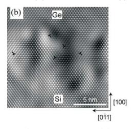
Figure 4. Cross-section TEM ima-ge of the Ge-Si interface.
