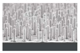
Figure 9. Si nanowires grown by use of a Al catalyst.
