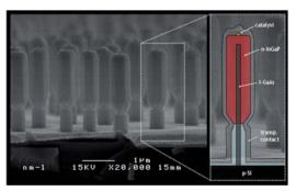
Figure 3. Nanowire array with light-emitting structures.
