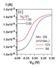
Figure 32. Sub-threshold I-V characteristics of an array of 55 vertical InAs nanowires.
