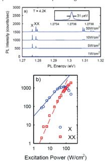
Figure 3. (a) Power dependence of the photoluminescence from a single quantum dot in a nanowire under continuous excitation at 532 nm. (b) Integrated power dependence of two narrow emission lines attributed to the exciton and biexciton. Samples grown by the Bakkers group.
