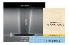
Figure 22. Cross-section of a via hole after plasma etch and hot phosphor opening of the  $Si_3N_4$  bottom layer.
