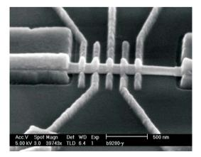
Figure 16. Horizontal InAs/InP nanowire with multiple gates.
