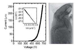
Figure 9. Left, the x-ray tube current versus the gate voltage measured with the anode voltage fixed at 40 kV. It follows the classic Fowler–Nordheim relation. The distance between the cathode and the gate is 150 μm. Right, X-ray image of a normal mouse carcass (25 g) obtained using a CNT source-based imaging system [158]. Reprinted with permission from J Zhang, Rev. Sci. Instrum. 76, 094301 (2005). Copyright 2005, American Institute of Physics.
