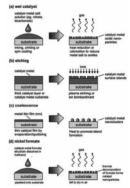
Figure 2. Methods of producing nano-sized catalysts for nanotube growth [13-16].
