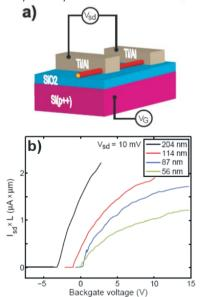
Figure 2. (a) Schematic of a Ti/Al contacted nanowire on a heavily doped Si substrate with SiO2 dielectric. (b) Current through the nanowire as a function of backgate voltage for several NW diameters. Such measurements are used to determine the electron mobility.
