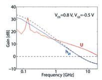
Figure 33. Measured and modelled RF gains for a 90 nm gate length InAs MOSFET.
