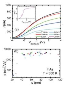
Figure 24. (a) the backgate sweeps for different sections within the same nanowire. The inset shows the data for the section with the smallest diameter. (b) the mobility determined from backgate sweeps. Different symbols correspond to the different devices studied.
