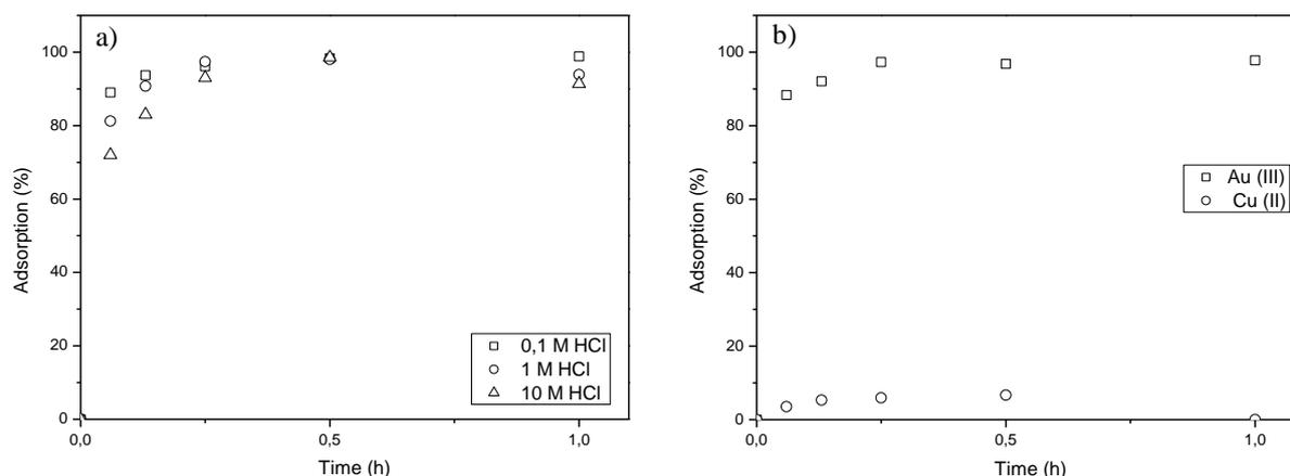
**Figure 1.- a)** Influence of the HCl concentration in the adsorption of Au (III), conditions; adsorbent dosage: 0.025 g (CN), aqueous phase: 0.05 g/l Au (III), temperature=20°C, stirring speed: 2000 cm<sup>-1</sup>. **b)** Mixture of gold (III) and copper (II), conditions; adsorbent: 0.1 g (CN), aqueous phase: 0.05 g/L Au (III) and 0.016 g/L Cu (II) in 6 M HCl, temperature 20°C, stirring speed: 2000 cm<sup>-1</sup>.
