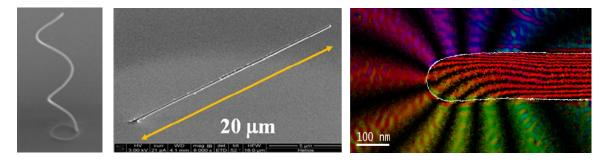
**Figure caption.** *Left.* Two-loop three-dimensional cobalt nanowire grown by FEBID. *Middle*: High aspect-ratio three-dimensional cobalt nanowire grown by FEBID. *Right*: Magnetic signal obtained in the electron holography experiments performed in one of the cobalt nanowires grown by FEBID.
