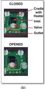
**Figure 1: (a)** Pictures of polyaniline functionalised PDMS chips, acidic on the top and basic on the bottom, as pH sensor. **(b)** Picture of an ionogel microvalve (7  $\mu$ L) inserted in the holder with integrated heaters at the bottom for fluid control.
