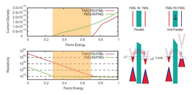
Fig. 1. Emergence of giant resistance in FMG/FEI heterojunctions. The blockade of quantum tunneling through the heterojunction originates from the anti-parallel configuration of FMGs.
