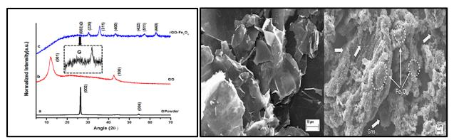
Fig. (a) XRD of rGO-Fe<sub>3</sub>O<sub>4</sub> nano composite (b) SEM of graphene oxide and rGO-Fe<sub>3</sub>O<sub>4</sub> nano composite
