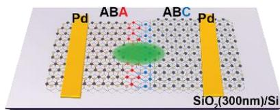
Figure 1 Schematic of ABA/ABC photodevice
