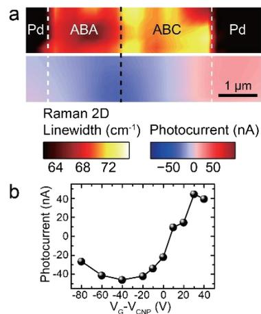
Figure 2 (a) Raman and photocurrent image of ABA/ABC photodevice (b) Gate bias dependence of photocurrent at the lateral ABA/ABC junction
