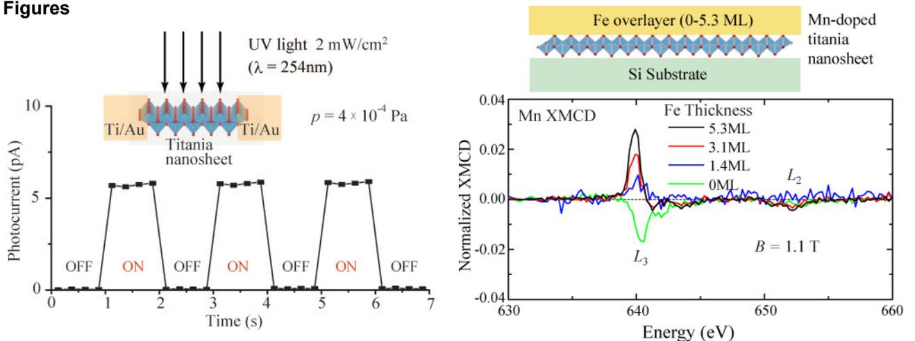
Figure 1: Photocurrent under periodic pulsed UV illuminations at bias voltage of 1.0 V.
