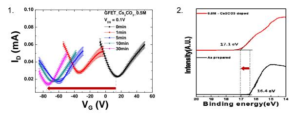
Figure 1. Transfer curves of  $Cs_2CO_3$  doped GFETs depending on the doping time Figure 2. UPS spectra of graphene before and after doping
