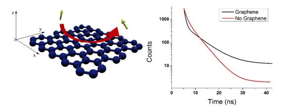
A schematic of the excitation transfer between molecular dipoles via the plasmonic waves excited in a nearby graphene sheet (left figure); Fluorescence decays curves for high concentrations of perylene molecules in a thin PMMA film (less that 2 nm) on top of or away from a single layer graphene flake. The increased emission at time scales of several nominal lifetimes of perylene is taken as evidence of the excitation transfer process.
