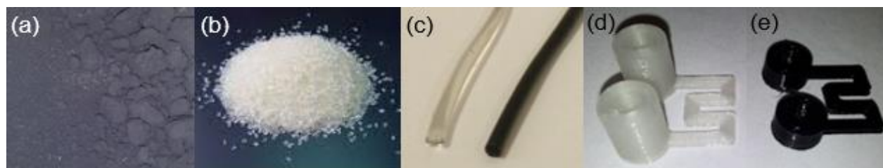
Figure 1: (a) Graphene Powder, (b) PLA pellets (c) Filament of PLA (White) and Graphene-PLA (Black), (d) Printed structure with pure PLA and (e) graphene-PLA composite.
