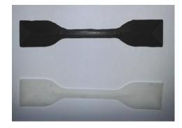
b) Tensile test samples manufactured by 3D printing
