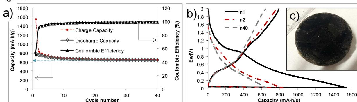
**Figure 1.** a) Charge/discharge curves and b) galvanostatic cycling of c) 3D-Sn/SnO<sub>2</sub>@rGO electrode.
