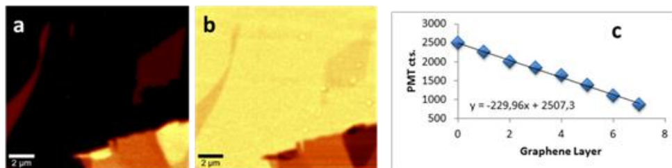
Fig. 1: Raman SNOM study of graphene: intensity of Raman G band (a), SNOM image (b), and decrease of transparency of graphene as a function of number of layers.
