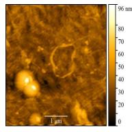
**Fig. 1a:** AFM image showing an isolated island formed by wrinkling. The height scale bar is in nm.
