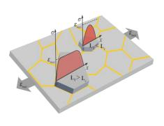
**Fig.1c**: Graph explaining the proposed stress transfer mechanism ( $L_i$  is the length of the *i*-crystallite and  $L_c$  the critical transfer length)
