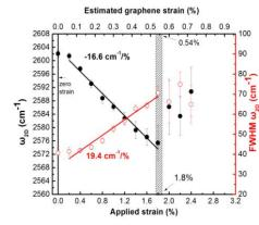
**Fig. 1b:** Pos(2D) and the corresponding FWHM(2D) as a function of the applied and the extracted actual strain for the graphene membrane on the PET substrate
