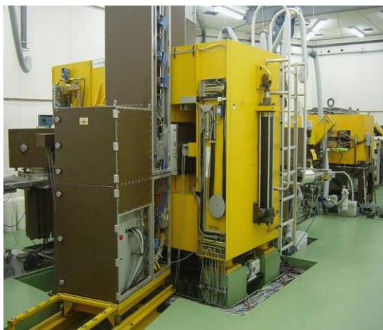
Figure 1: The Scanditronix MC-40 Cyclotron at JRC Ispra, and the target capsule and holder used for direct ion-beam radiolabelling of dry nano-particulate powders.
