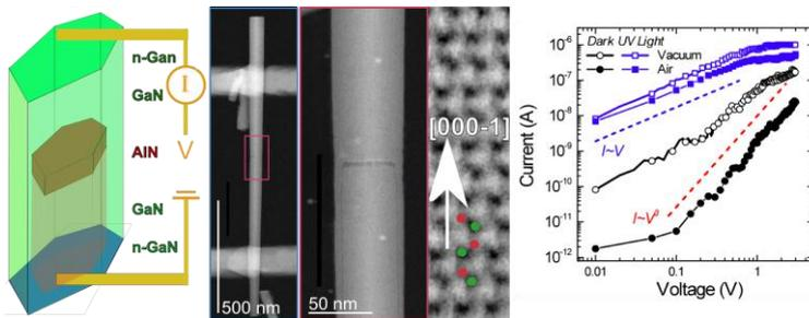
Fig. 1. From left to right: schematic of the NW structure, HAADF STEM image of a contacted GaN NW with an AlN insertion. Zoom of the boxed region viewed along the  $[11\bar{2}0]$  direction. Atomic structure of GaN viewed along  $[11\bar{2}0]$  overlaid on an ABF STEM image.  $I$ - $V$  characteristic from *the same* NW device measured in the air and in vacuum, in the dark and under UV illumination.
