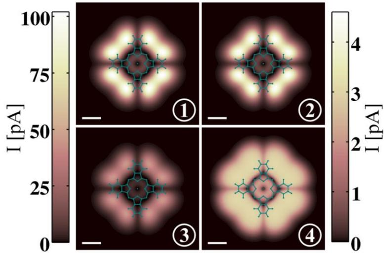
**Fig. 2** Constant-height current maps calculated for different bias voltages. The color bar on the left (right)-hand side corresponds to maps 1 and 3 (maps 2 and 4). The current map in the interference blockade regime (map 4) appears to be flat in the molecule region.
