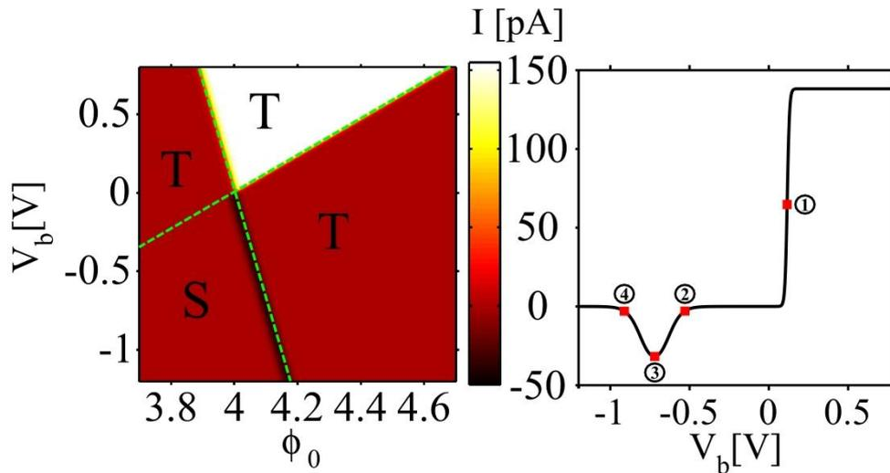
**Fig. 1:** Left: Current through a CuPc singlemolecule junction as a function of the substrate (and tip) work function  $\phi_0$  and of the sample bias  $V_b$ . Right: Current obtained from a cut of the left-hand plot corresponding to  $\phi_0 = 4.1$  eV. The current scale is the same for the left and right panels. The numbers in the current-voltage plot refer to the current maps in Fig. 2 and Fig. 3.
