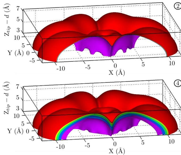
**Fig. 3** Isosurfaces of constant current calculated in the proximity of the Coulomb blockade (upper panel;  $V_b = 0.5303$  V) and interference blockade (lower panel;  $V_b = -0.9118$  V) regimes. The surfaces correspond, in both cases, to the currents:  $I = 3.15, 3.075, 3.0, 2.925,$  and  $2.85$  pA.
